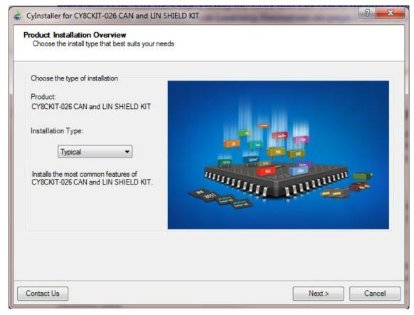
6. Read and accept the End-User License Agreement and click Next to proceed with the installation. After the installation is complete, the kit contents are available at the following location: C:\Program Files (x86)\Cypress\CY8CKIT-026 CAN and LIN SHIELD KIT\<version>
