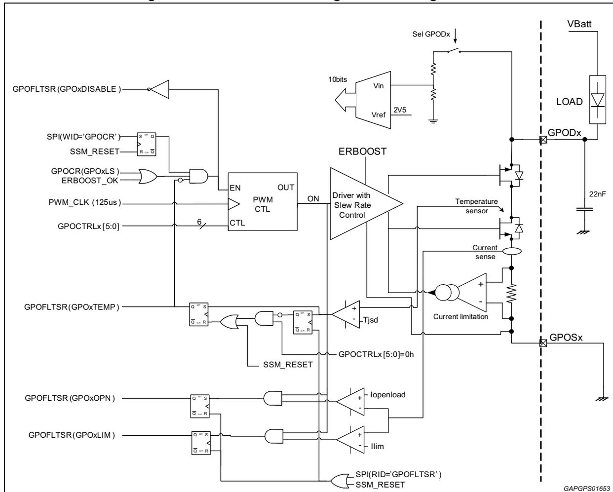
For high side driver configuration, the GPODx pin will be connected to battery and GPOSx pin will be connected to the load high side.
