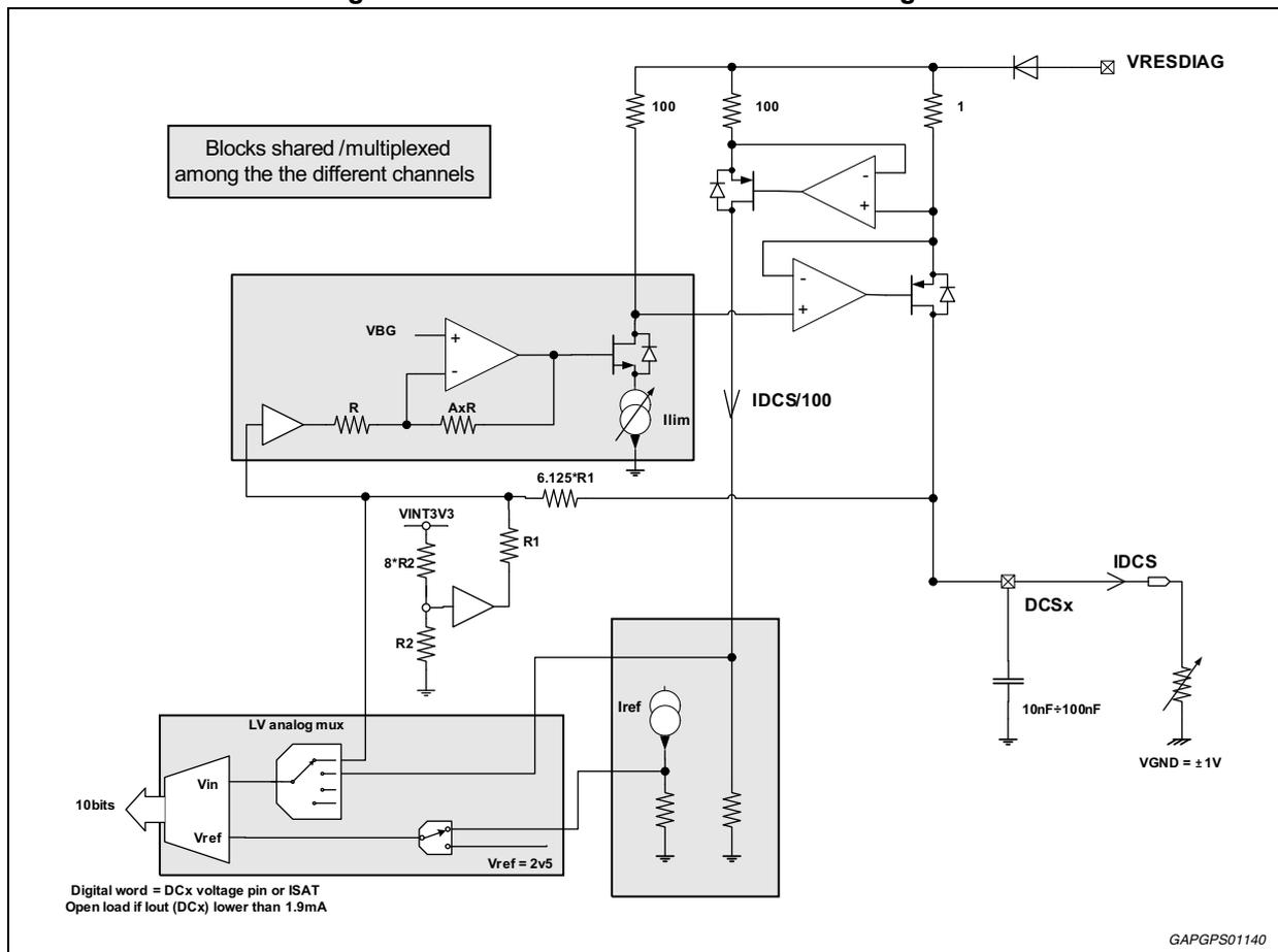
The global SPI contains several bits to control and configure the interface. The SWOEN bit is used to enable the output voltage on DCSx pins. The channel to be activated can be chosen by setting CHID bits accordingly. The interface activation is completely controlled by user SPI command. The interface could be optionally configured for "automatic switch-off" immediately after the current or resistance measurement completion by setting the EN\_AUTO\_SWITCH\_OFF bit in the SYS\_CFG register.
