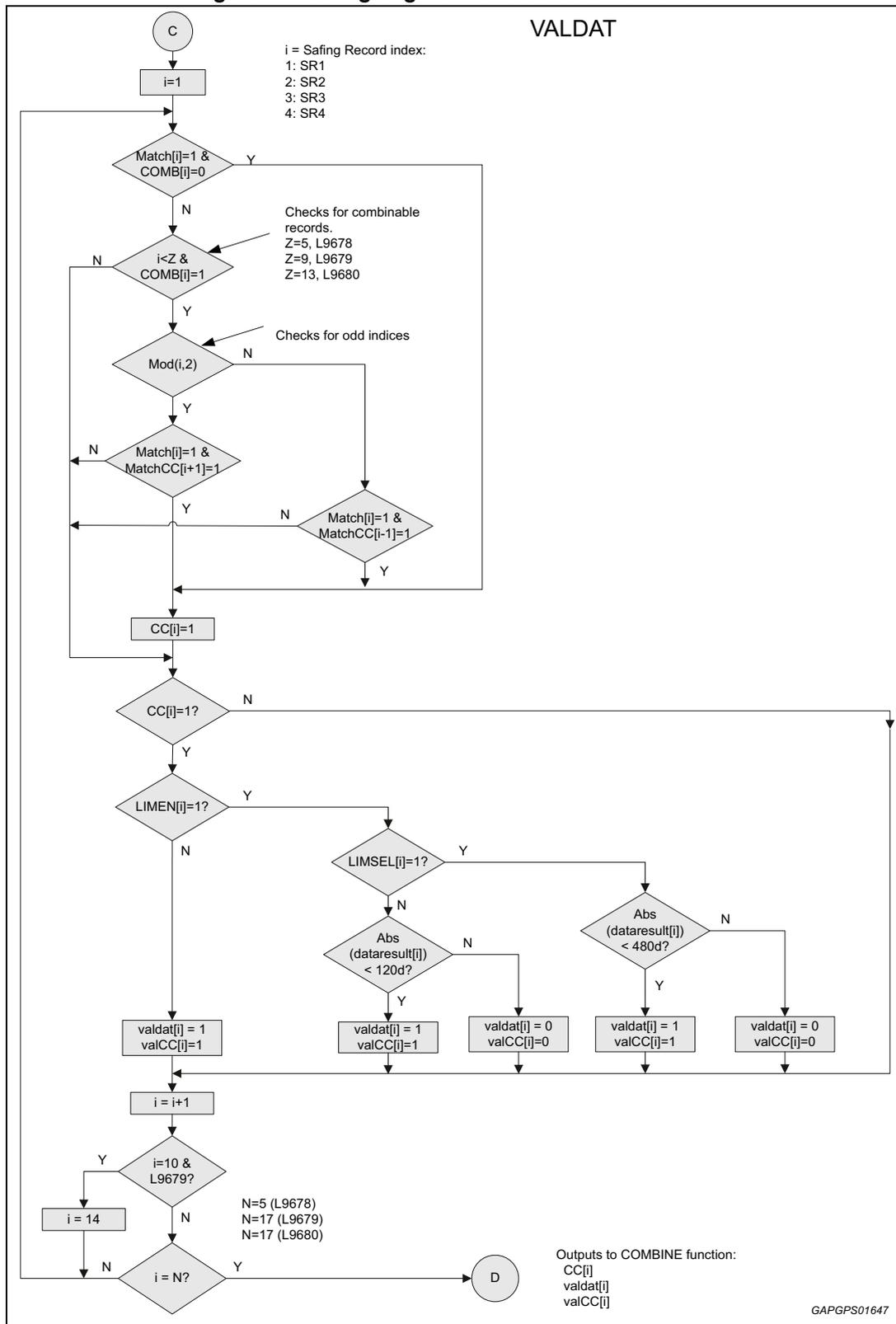
Figure 43. Safing engine - combine function flow chart
