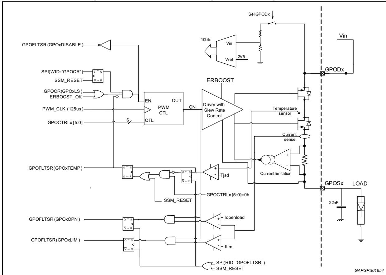
The drivers have to be configured in one of the two modes through the GPO Configuration Register (GPOCR) register before being activated. This hardware configuration is only allowed during the Init and Diag states.
