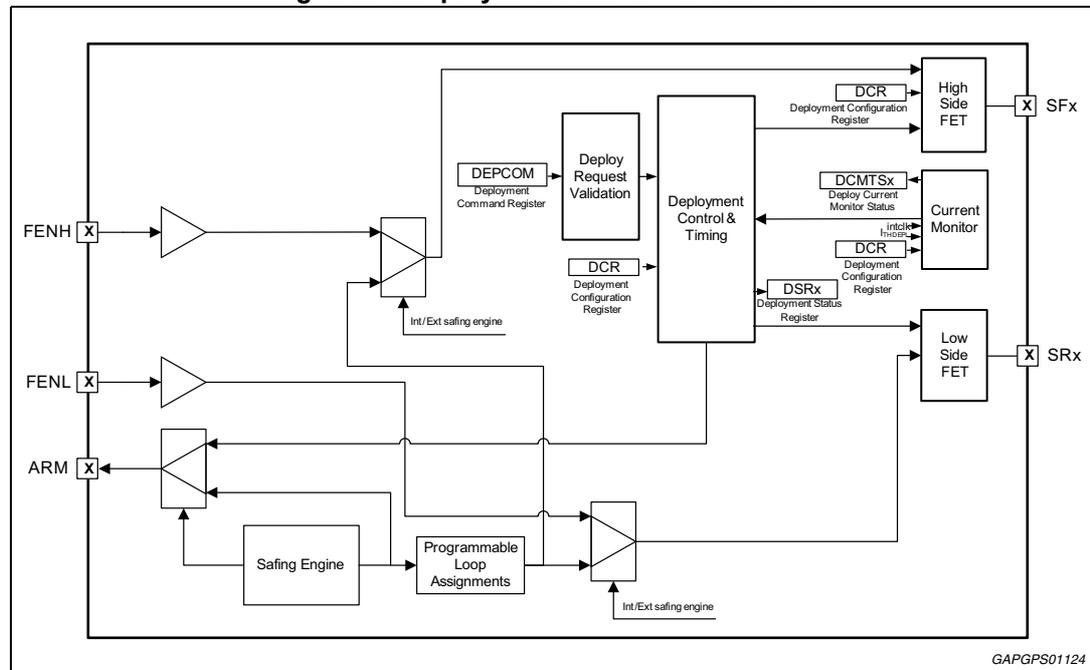
Figure 21. Deployment driver control logic - Enable signal
