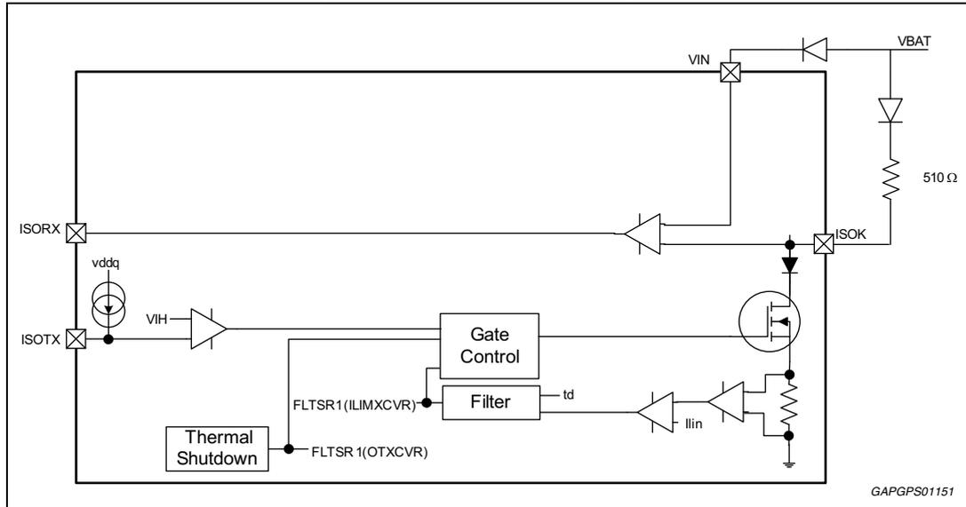
When the ISOTX pin is asserted, logic high, the ISOK output will be disabled (pulled high by an external resistor). When the ISOTX pin is deasserted, logic low, the ISOK output will be enabled (pulled low by the internal driver). This input pin contains an internal pull-up to command the output to the disabled state in the event of an open circuit condition.
