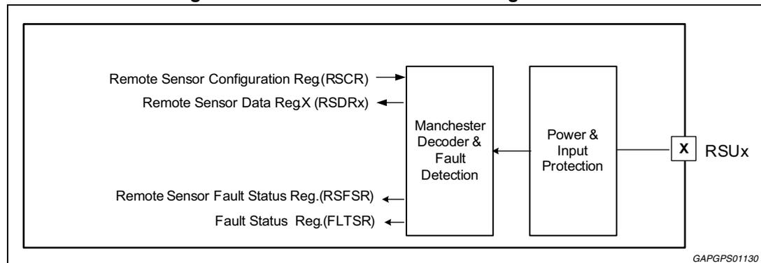
The Remote Sensor Configuration Registers (RSCRx) allow for configuration of the particular PSI5 protocol adopted by the sensor and the transceiver current limit blanking time.
