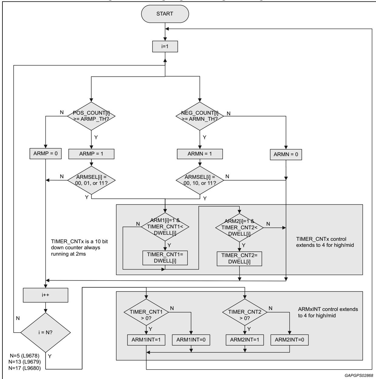
Figure 49. Safing engine diagnostic logic
