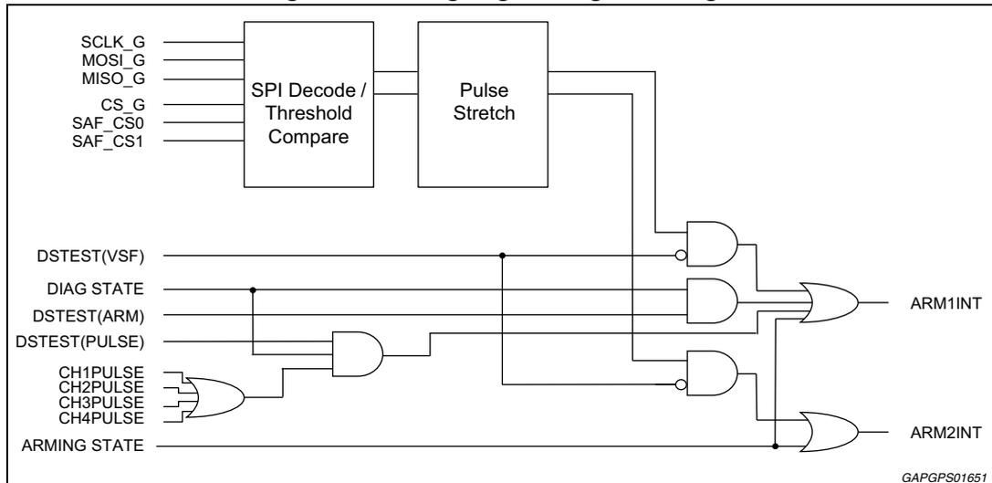
A configurable mask for each internal ARMxINT signal is available for all of the integrated deployment loops (refer to [ARMx assignment registers \(LOOP\\_MATRIX\\_ARMx\) on page 97](#)). The un-masked ARMxINT signal for each loop will enable the respective loop drivers (refer to [Figure 21](#)).
