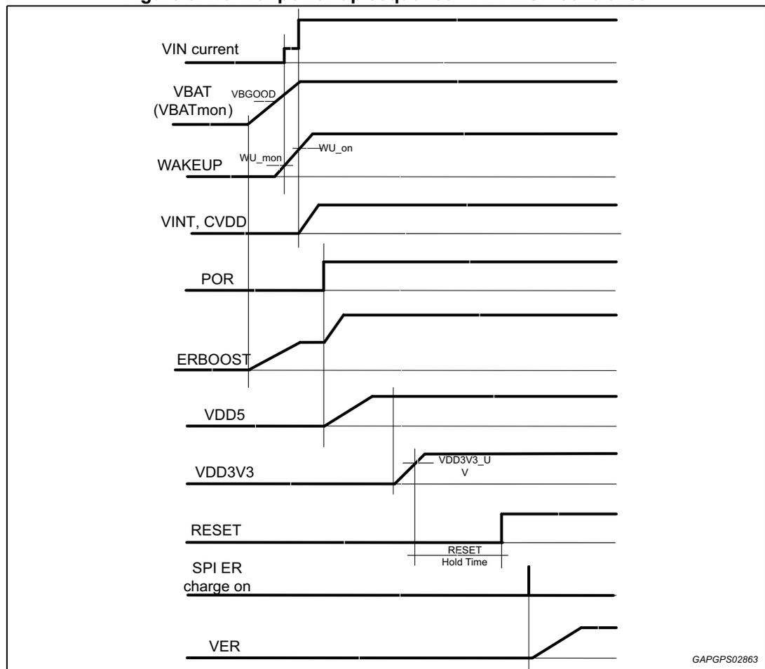
Figure 6. Normal power-up sequence - VIN controlled
