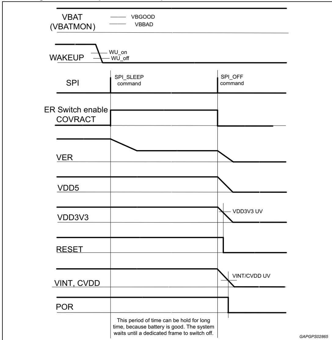
Figure 8. Normal power down sequence - VIN controlled
