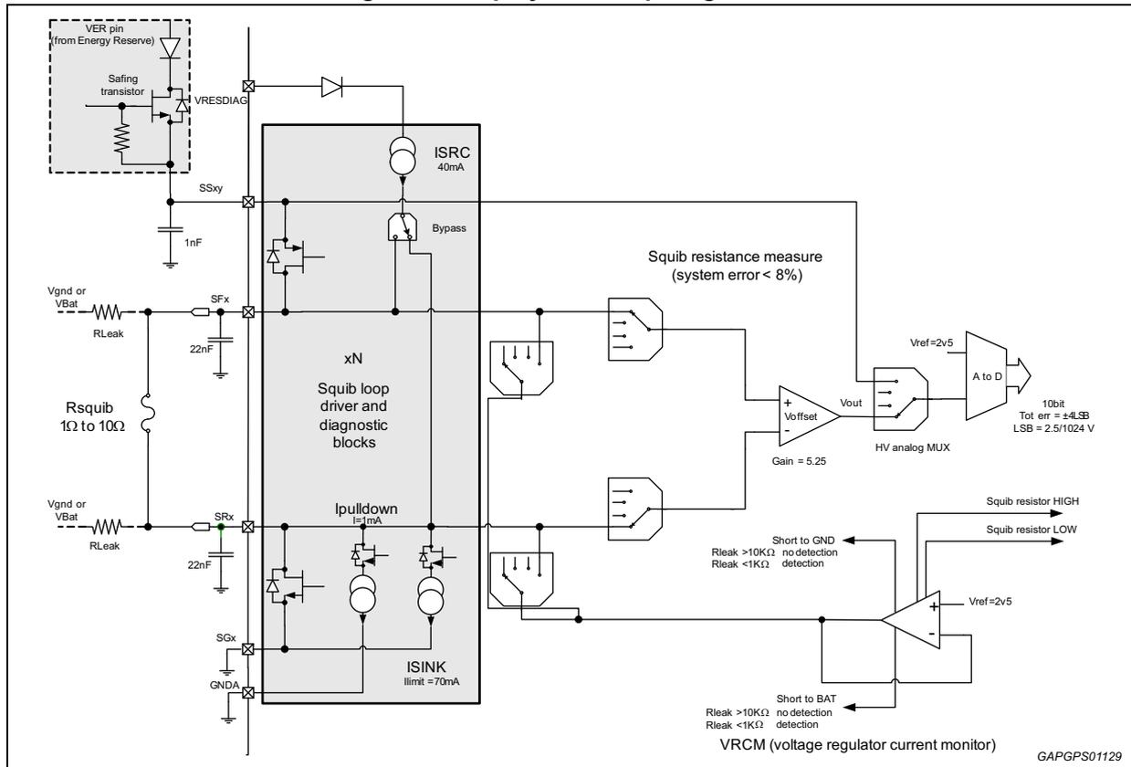
The leakage diagnostic includes short to battery, short to ground and shorts between loops. The test is applied to each SFx and SRx pin so shorts can be detected regardless of the resistance between the squib pins.
