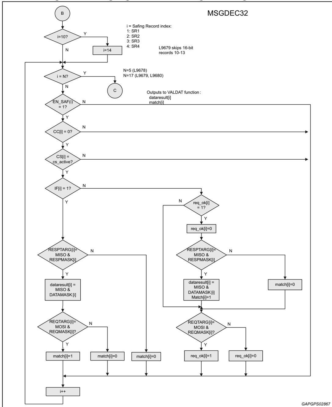
Figure 42. Safing engine - validate data flow chart
