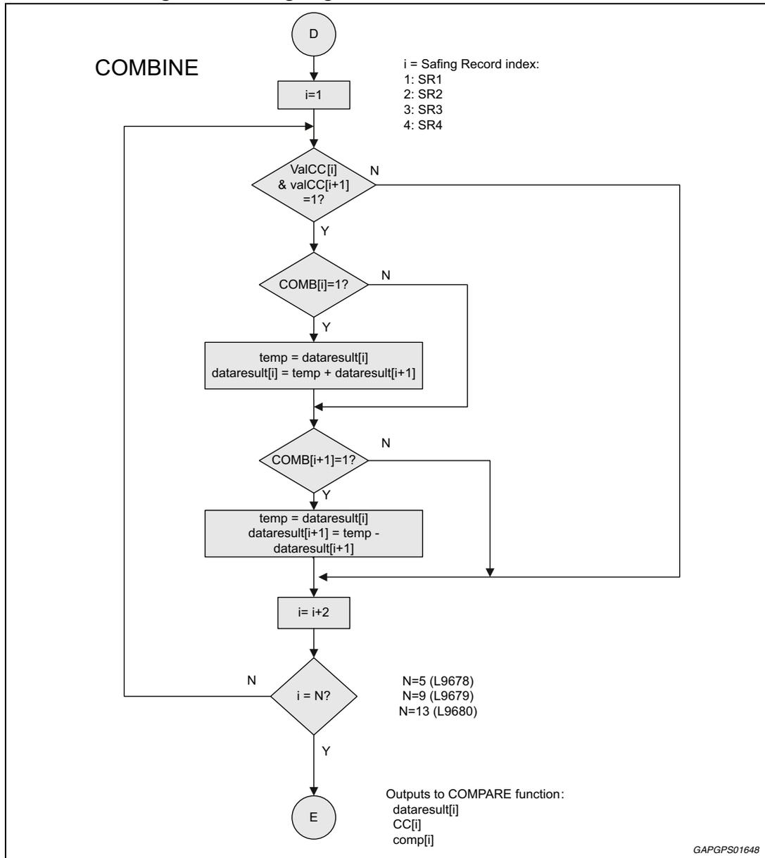
Figure 44. Safing engine threshold comparison
