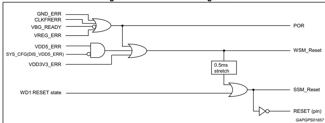
GND\_ERR is a general fault signal with the purpose of driving the device into POR when either GNDA or GNDD is shifted more than 300 mV nominal with respect to the reference ground pins GNDSUB.
