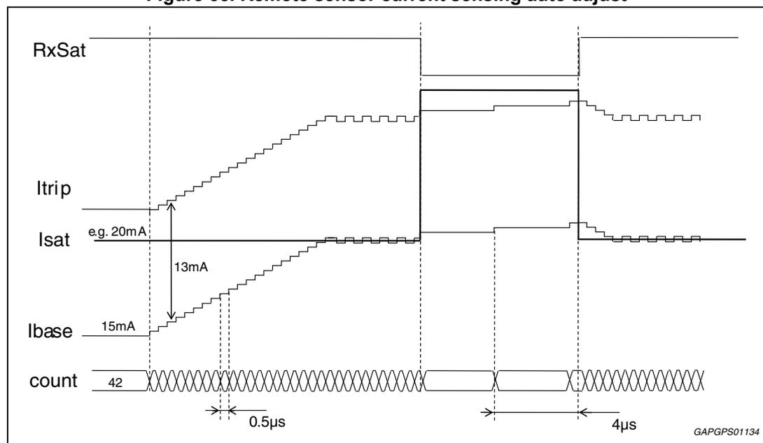
The auto adjust feature uses a 7 bit D/A to converter to step up and down the threshold level for detecting the base current through the remote sensor before start bits are transmitted. Once start bits are received, the counter stops and the D/A value remains fixed until the remote sensor message is received. This procedure is repeated for each cycle of the remote sensor. The auto adjust circuit uses the following equation:
