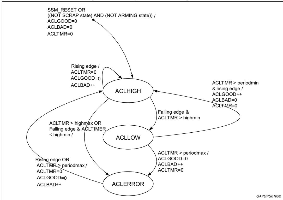
A specific waveform needs to be present on this input in order to instruct L9678P to arm all deployment loops. L9678P is designed to support the Additional Communication Line (ACL) aspect of the ISO-26021 standard, which requires an independent hardwired signal (ACL) to implement the scrapping feature. The disposal signal may come from either the vehicle's service connector, or the systems main microcontroller, depending on the end customer's requirements.
