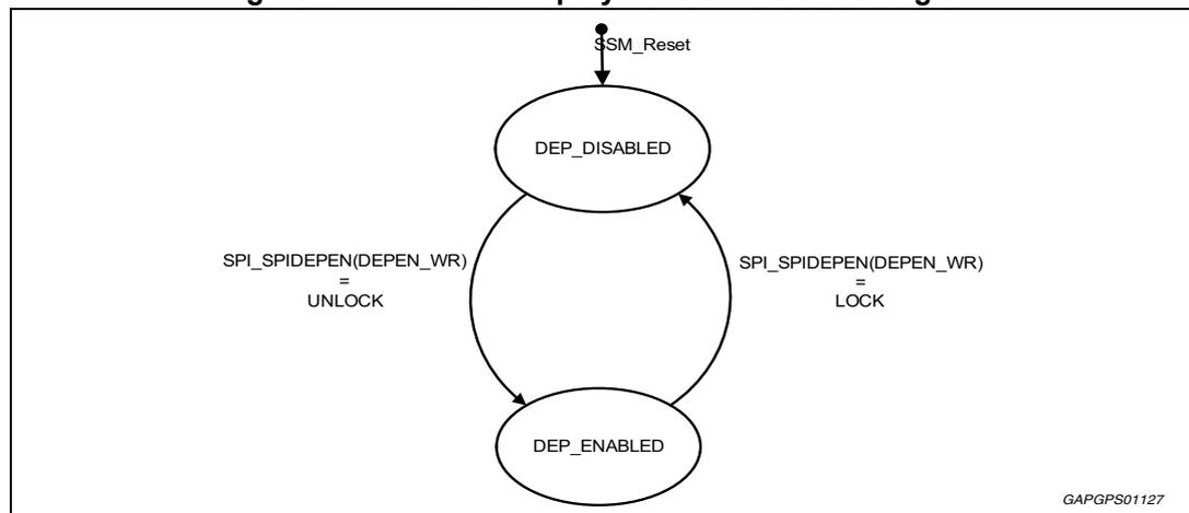
In case a multiple deployment request would be needed, i.e. deploying the same channel in sequence, a toggle on DEP\_DISABLED has to be performed and a new DEPCOM command on the same channel has to be sent.
