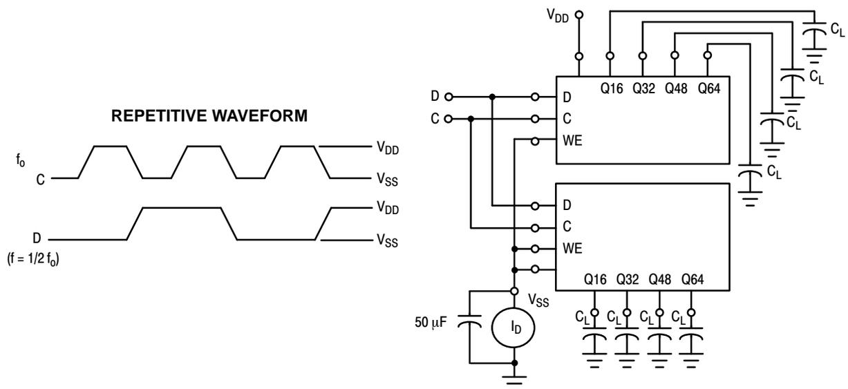
Figure 1. Power Dissipation Test Circuit and Waveform
