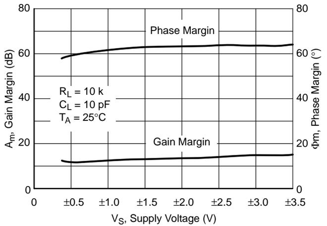
Figure 25. Gain and Phase Margin vs. Supply Voltage
