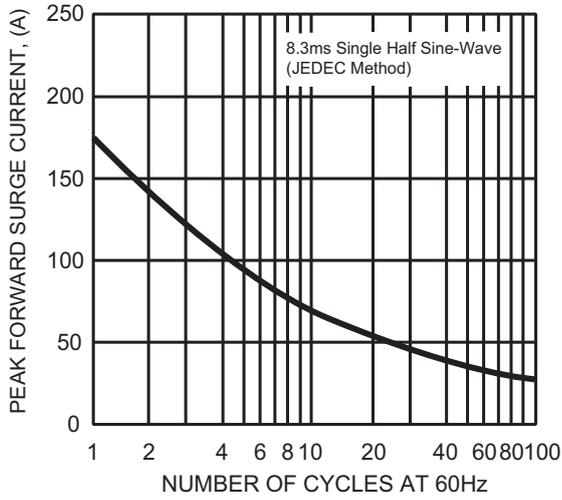
FIG. 2 - TYPICAL FORWARD CURRENT DERATING CURVE
