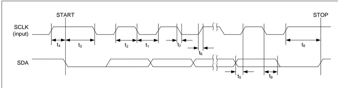
**Figure 4 Control Interface Timing – I<sup>2</sup>C Control Mode**
