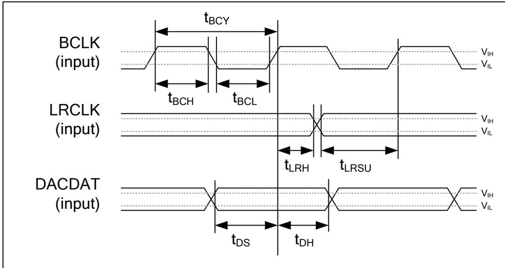
**Figure 3 Digital Audio Data Timing – Slave Mode**
