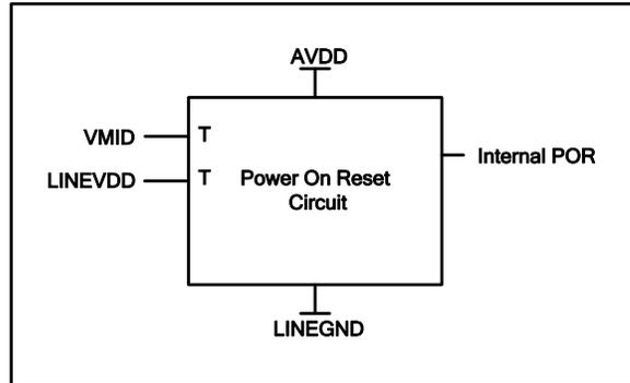
**Figure 6 Internal Power on Reset Circuit Schematic**
