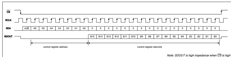
**Figure 13 SPI Control Interface – read operation**
