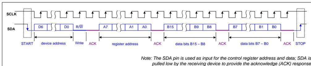
**Figure 8 Control Interface I<sup>2</sup>C Register Write**
