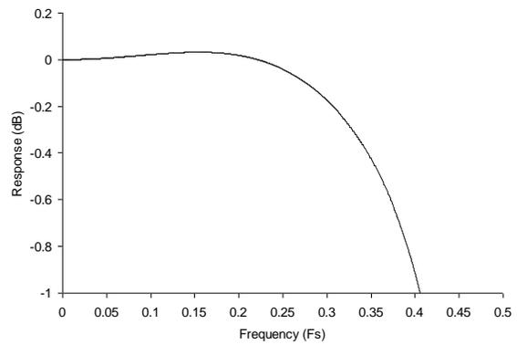
**Figure 30 DAC Digital Filter Ripple – 128fs to 192fs Clock Modes**
