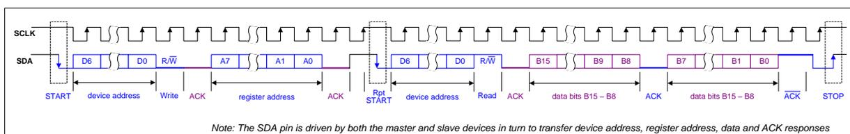
**Figure 9 Control Interface I<sup>2</sup>C Register Read**
