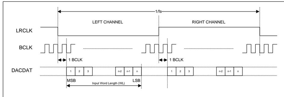
**Figure 18 I<sup>2</sup>S Justified Audio Interface (assuming n-bit word length)**
