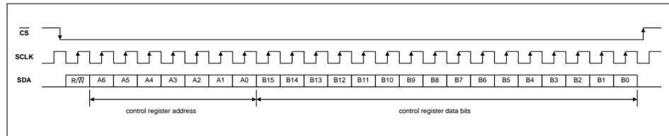
**Figure 12 SPI Control Interface – write operation**
