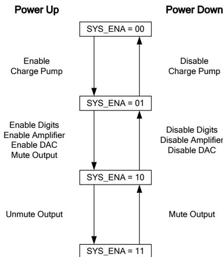
**Figure 23 SYS\_ENA[1:0] Power Up and Down Sequences**
