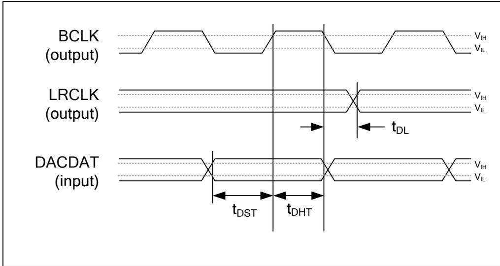
**Figure 2 Master Mode Digital Audio Data Timing**
