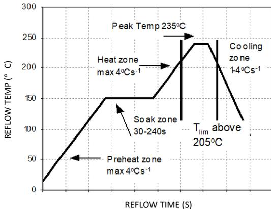
Figure 22. Reflow Profile for Tin/Lead (Sn/Pb) process.
