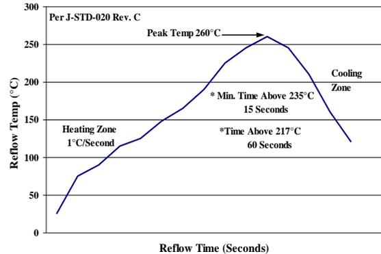
Figure 24. Recommended linear reflow profile using Sn/Ag/Cu solder.
