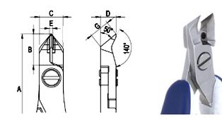
Tungsten Carbide Sharp Tip - Tapered Angled Cutters
