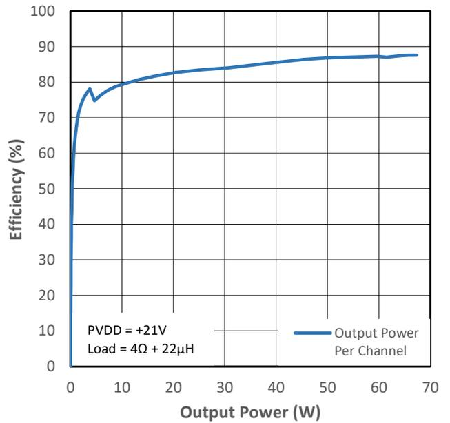
Figure 14-10 PMP1 Efficiency (VDD+PVDD) vs Output Power
