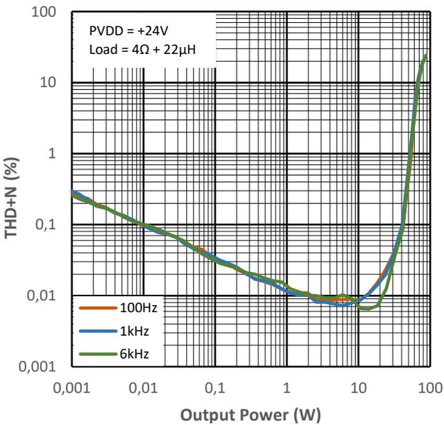
Figure 12-3 THD+N vs Output Power for PMP2
