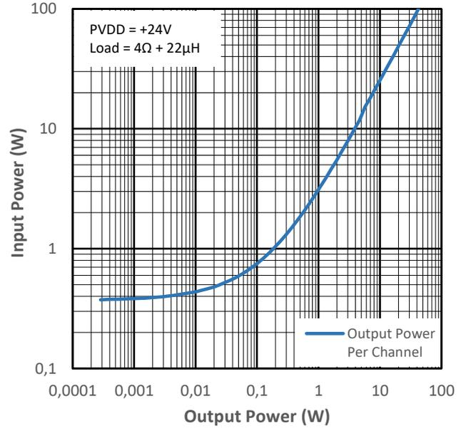
Figure 12-14 Input Power vs Output Power for PMP1
