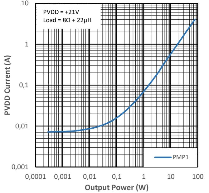
Figure 15-18 PVDD Current vs Output Power for PMP1
