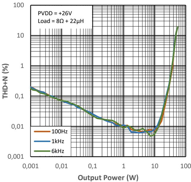
Figure 11-3 THD+N vs Output Power for PMP2
