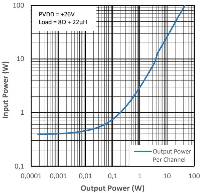
Figure 11-15 Input Power vs Output Power for PMP2
