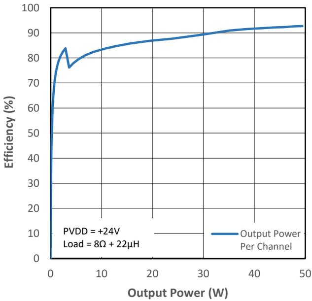
Figure 13-9 PMP0 Efficiency (VDD+PVDD) vs Output Power
