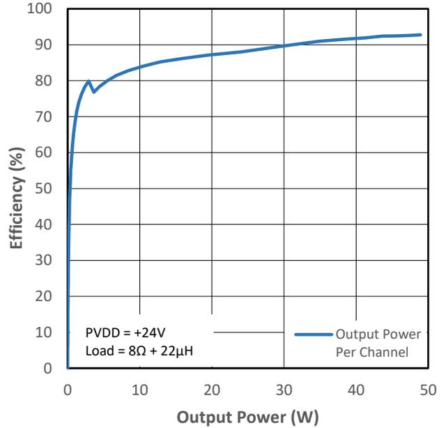
Figure 13-10 PMP1 Efficiency (VDD+PVDD) vs Output Power
