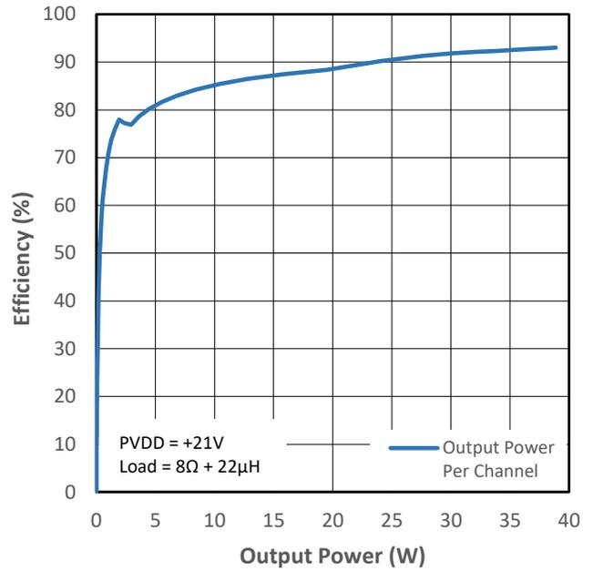
Figure 15-10 PMP1 Efficiency (VDD+PVDD) vs Output Power
