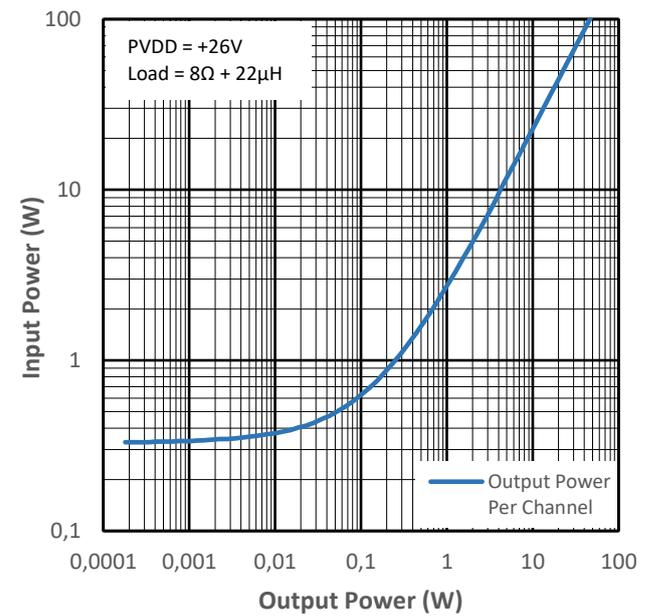
Figure 11-16 Input Power vs Output Power for PMP4
