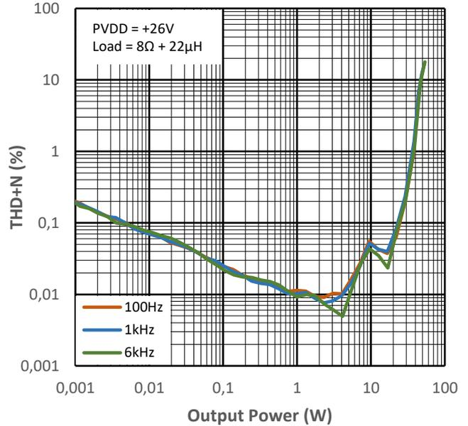
Figure 11-2 THD+N vs Output Power for PMP1
