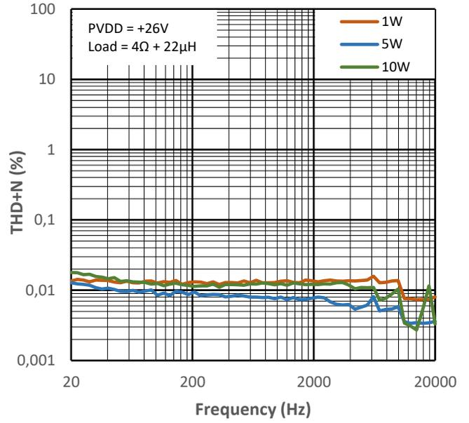
Figure 10-6 THD+N vs Frequency for PMP1
