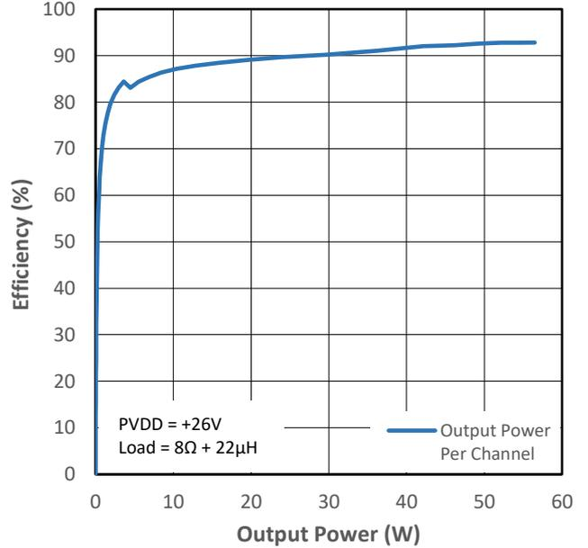
Figure 11-12 PMP4 Efficiency (VDD+PVDD) vs Output Power
