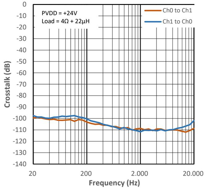
Figure 12-26 Crosstalk vs Frequency for PMP1
