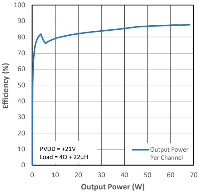
Figure 14-9 PMP0 Efficiency (VDD+PVDD) vs Output Power
