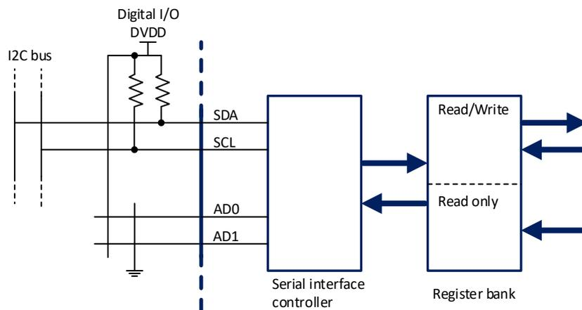
**Figure 8-7. I2C bus interface and register bank**
