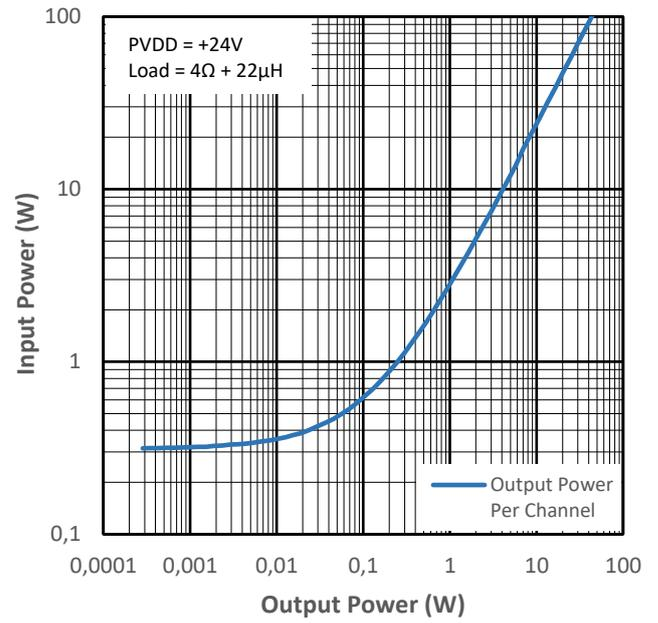
Figure 12-16 Input Power vs Output Power for PMP4
