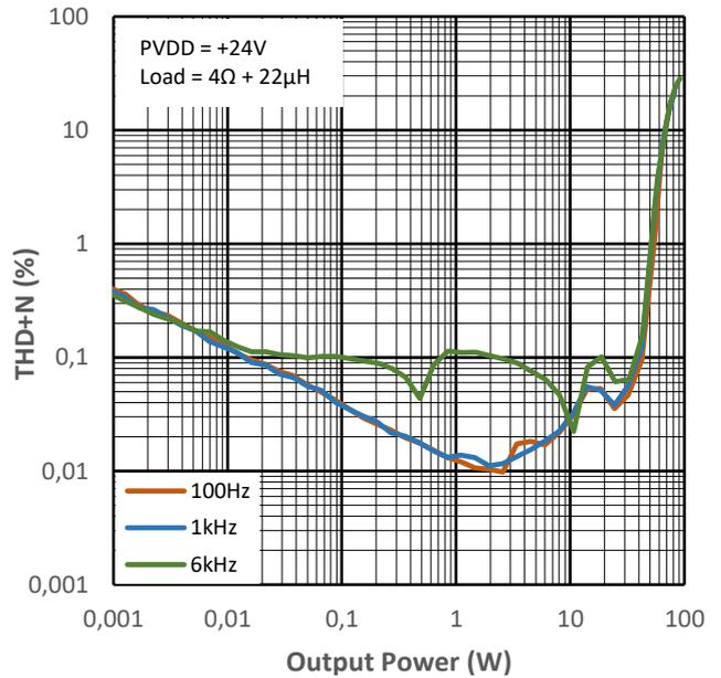
Figure 12-4 THD+N vs Output Power for PMP4
