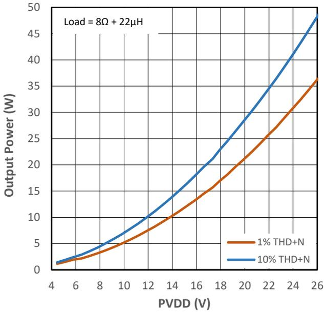
Figure 11-21 Output Power vs PVDD for PMP0
