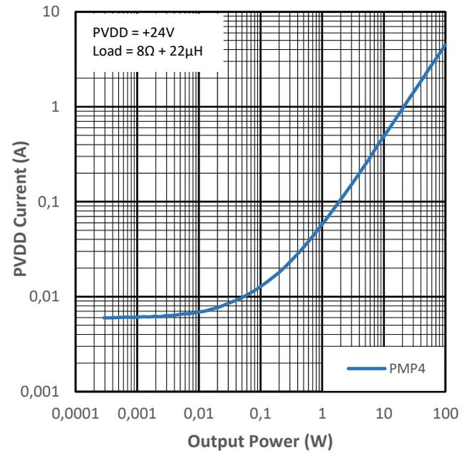
Figure 13-20 PVDD Current vs Output Power for PMP4
