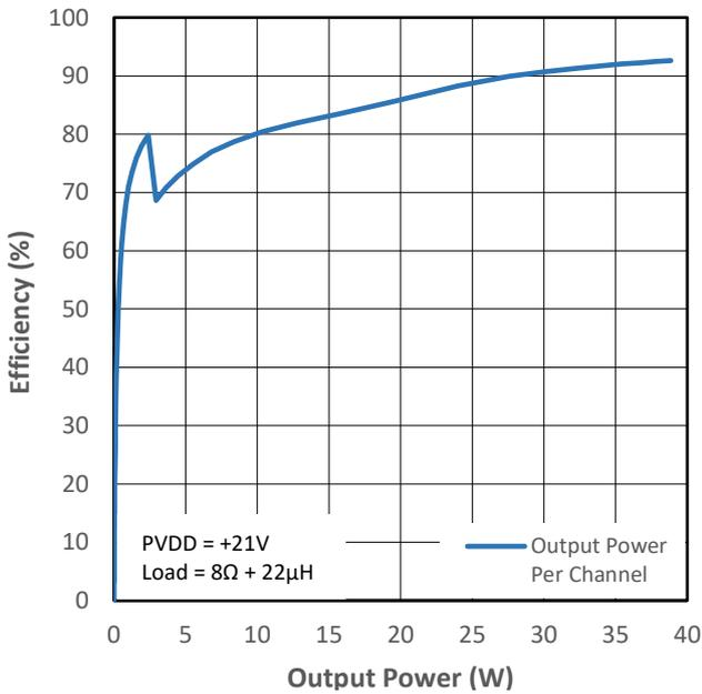
Figure 15-11 PMP2 Efficiency (VDD+PVDD) vs Output Power
