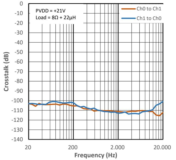
Figure 15-26 Crosstalk vs Frequency for PMP1
