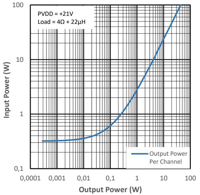
Figure 14-16 Input Power vs Output Power for PMP4
