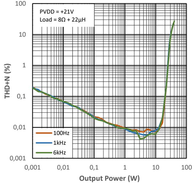
Figure 15-2 THD+N vs Output Power for PMP1
