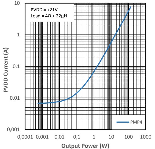
Figure 14-20 PVDD Current vs Output Power for PMP4
