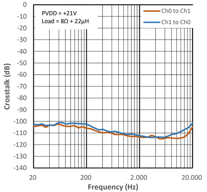
Figure 15-28 Crosstalk vs Frequency for PMP4
