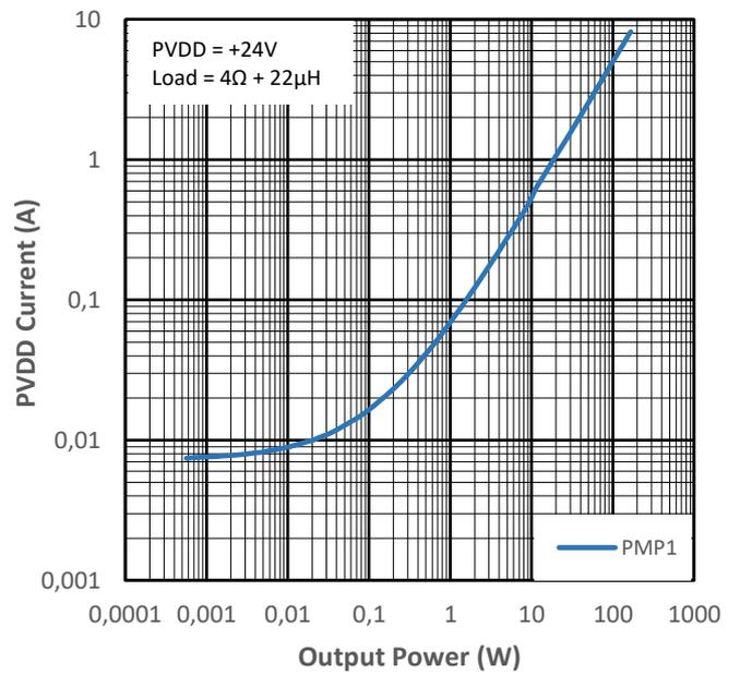
Figure 12-18 PVDD Current vs Output Power for PMP1
