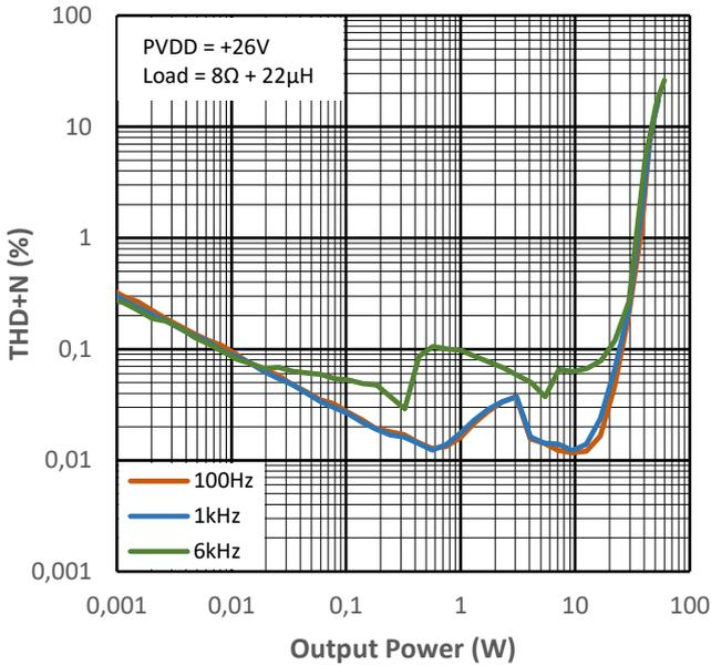
Figure 11-1 THD+N vs Output Power for PMP0
