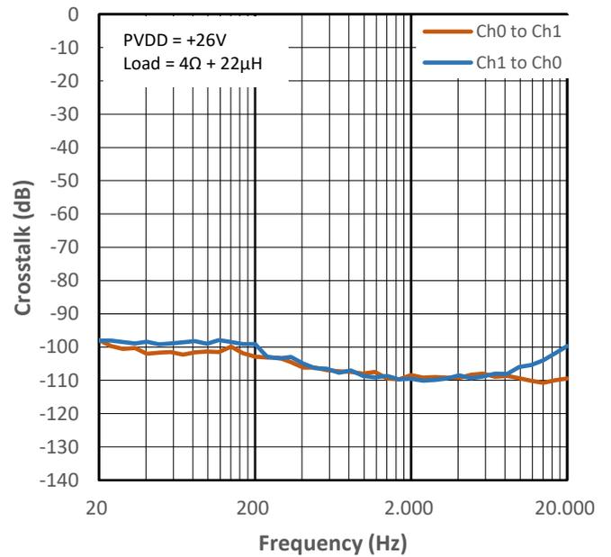
Figure 10-32 Crosstalk vs Frequency for PMP4
