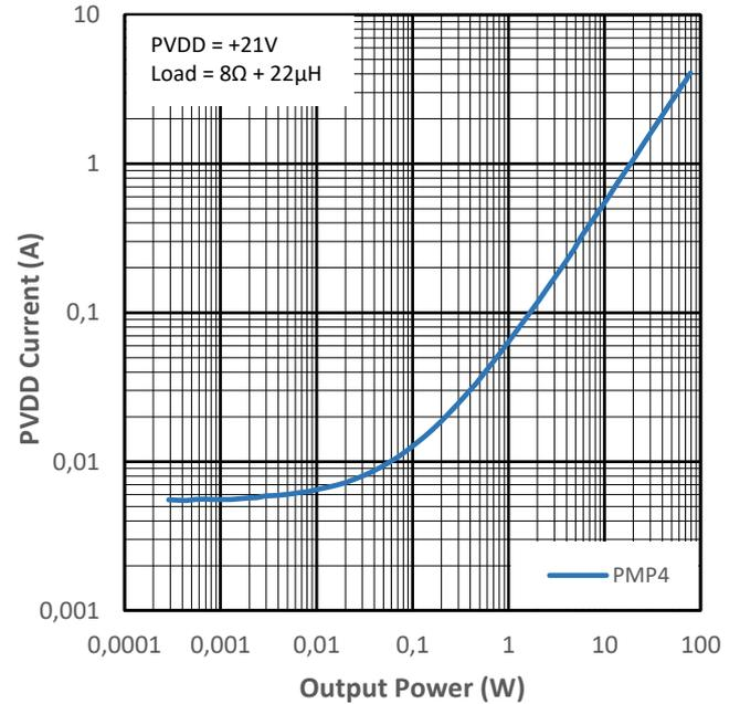
Figure 15-20 PVDD Current vs Output Power for PMP4
