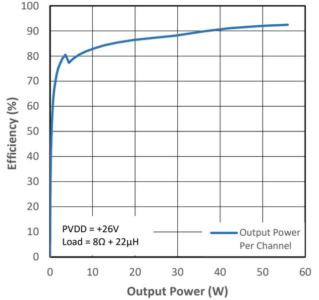
Figure 11-10 PMP1 Efficiency (VDD+PVDD) vs Output Power
