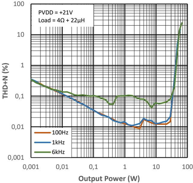
Figure 14-1 THD+N vs Output Power for PMP0
