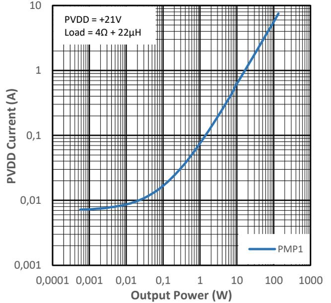
Figure 14-18 PVDD Current vs Output Power for PMP1
