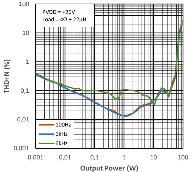
Figure 10-4 THD+N vs Output Power for PMP4
