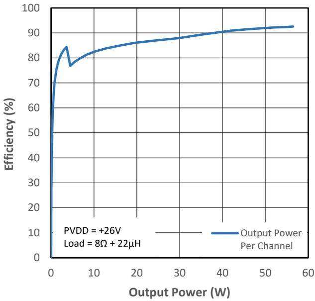
Figure 11-9 PMP0 Efficiency (VDD+PVDD) vs Output Power
