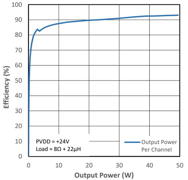
Figure 13-12 PMP4 Efficiency (VDD+PVDD) vs Output Power
