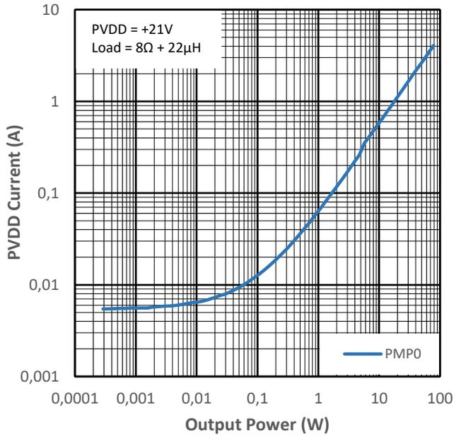
Figure 15-17 PVDD Current vs Output Power for PMP0
