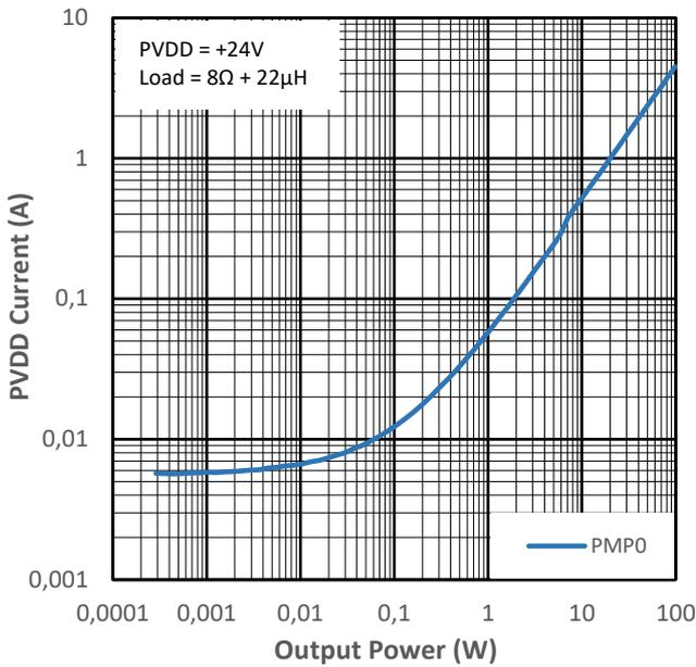
Figure 13-17 PVDD Current vs Output Power for PMP0
