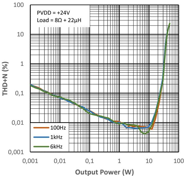
Figure 13-3 THD+N vs Output Power for PMP2
