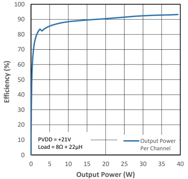
Figure 15-12 PMP4 Efficiency (VDD+PVDD) vs Output Power
