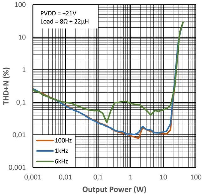
Figure 15-1 THD+N vs Output Power for PMP0
