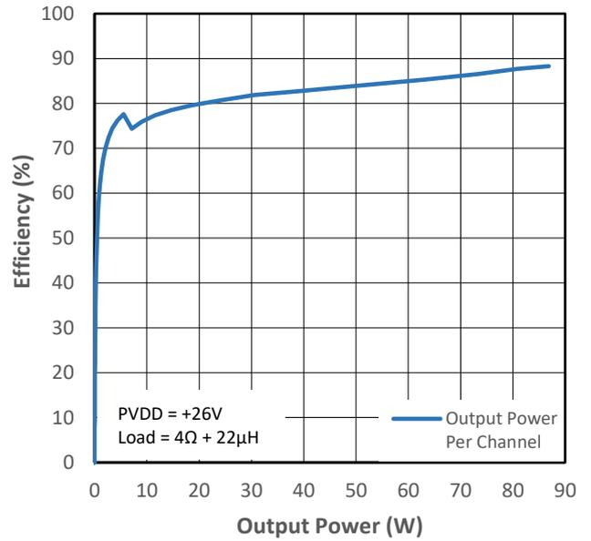
Figure 10-10 PMP1 Efficiency (VDD+PVDD) vs Output Power
