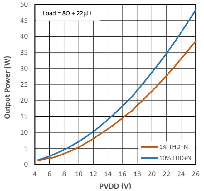
Figure 11-22 Output Power vs PVDD for PMP1
