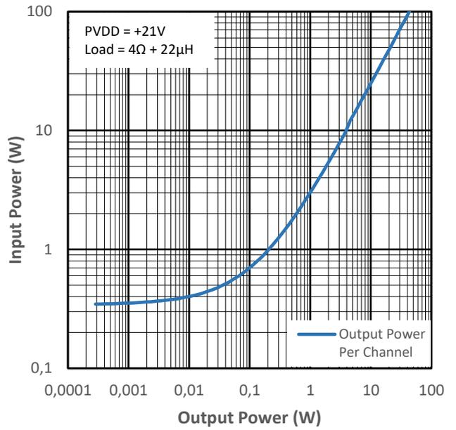
Figure 14-14 Input Power vs Output Power for PMP1
