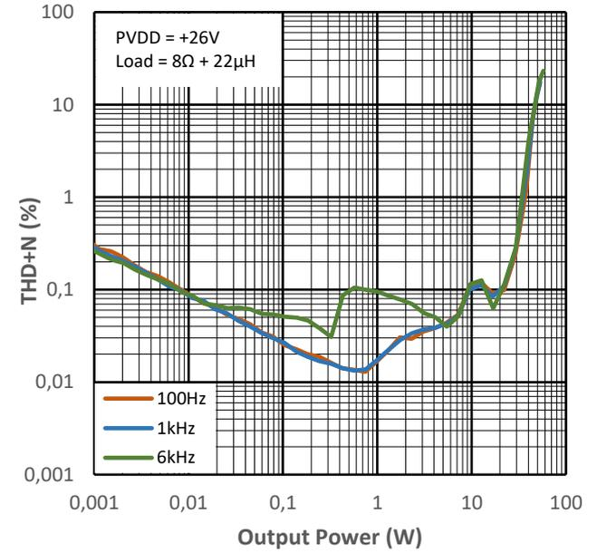
Figure 11-4 THD+N vs Output Power for PMP4
