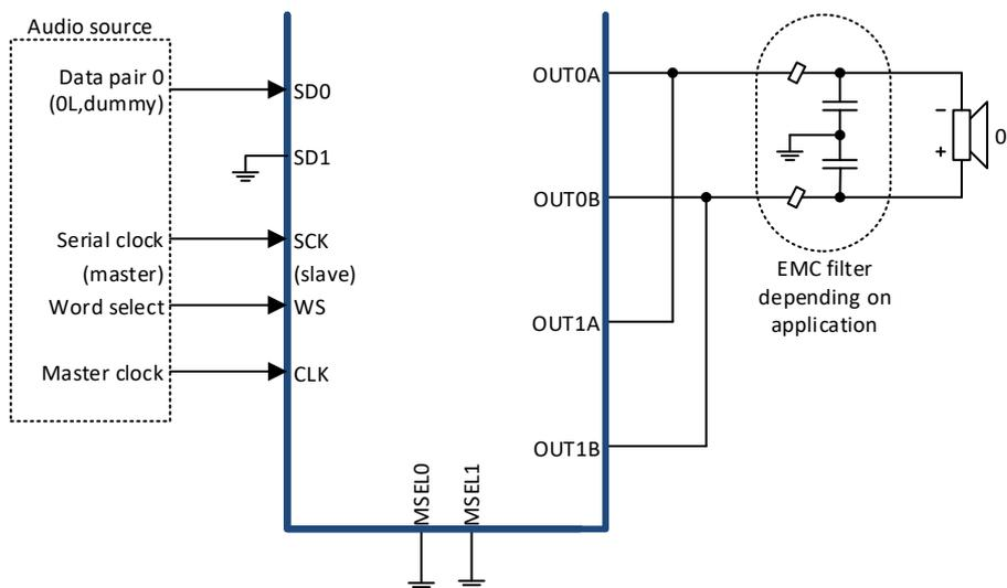
Figure 9-4 Parallel Bridge Tied Load (PBTL) configuration
