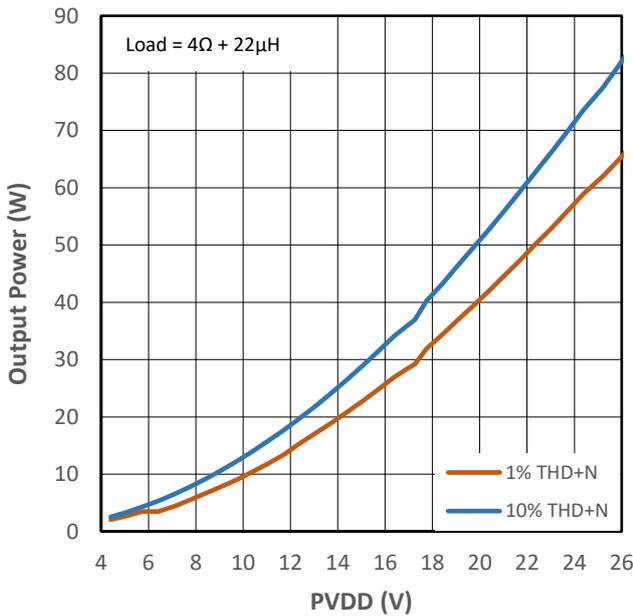
Figure 10-23 Output Power vs PVDD for PMP2
