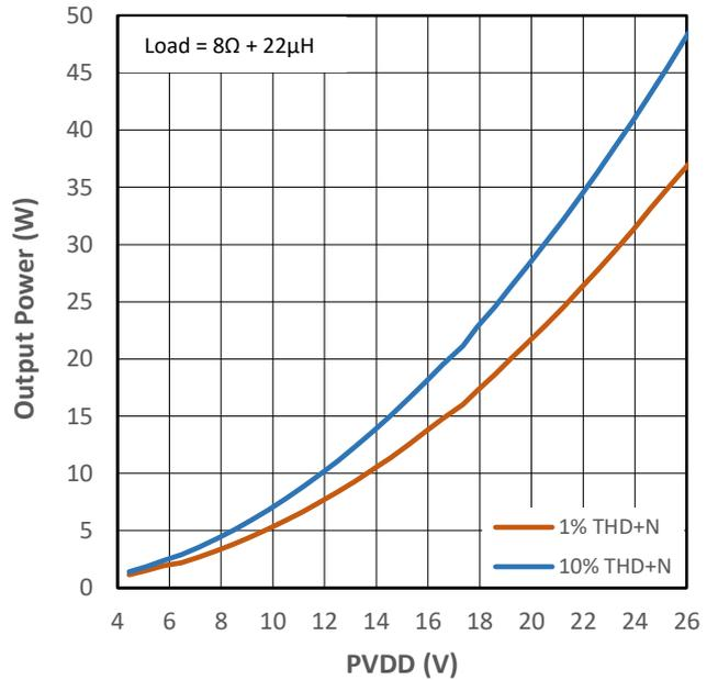
Figure 11-24 Output Power vs PVDD for PMP4
