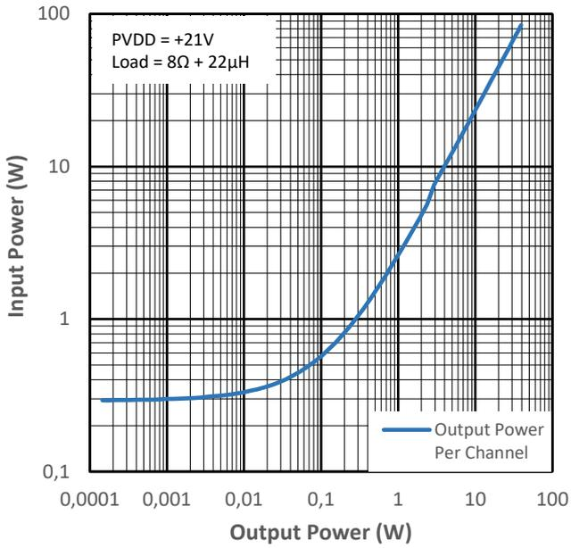
Figure 15-13 Input Power vs Output Power for PMP0
