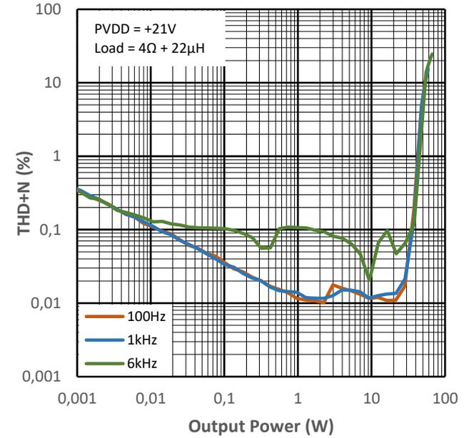
Figure 14-4 THD+N vs Output Power for PMP4
