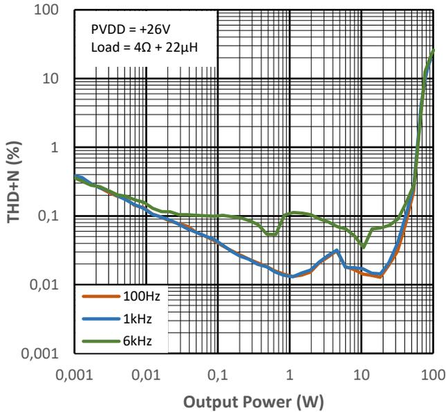
Figure 10-1 THD+N vs Output Power for PMP0
