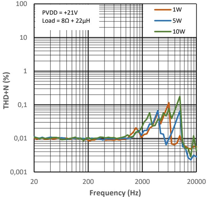
Figure 15-8 THD+N vs Frequency for PMP4
