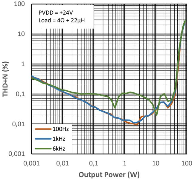
Figure 12-1 THD+N vs Output Power for PMP0
