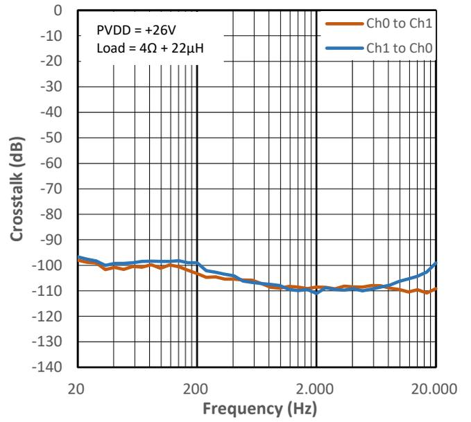
Figure 10-30 Crosstalk vs Frequency for PMP1
