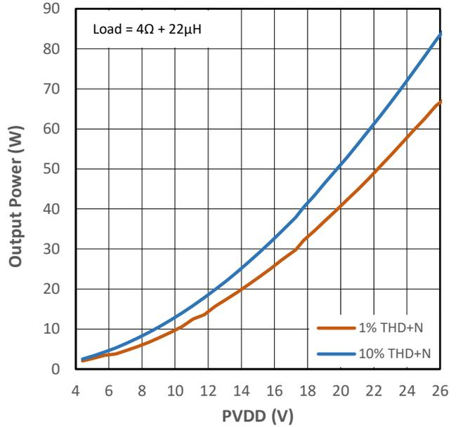
Figure 10-22 Output Power vs PVDD for PMP1
