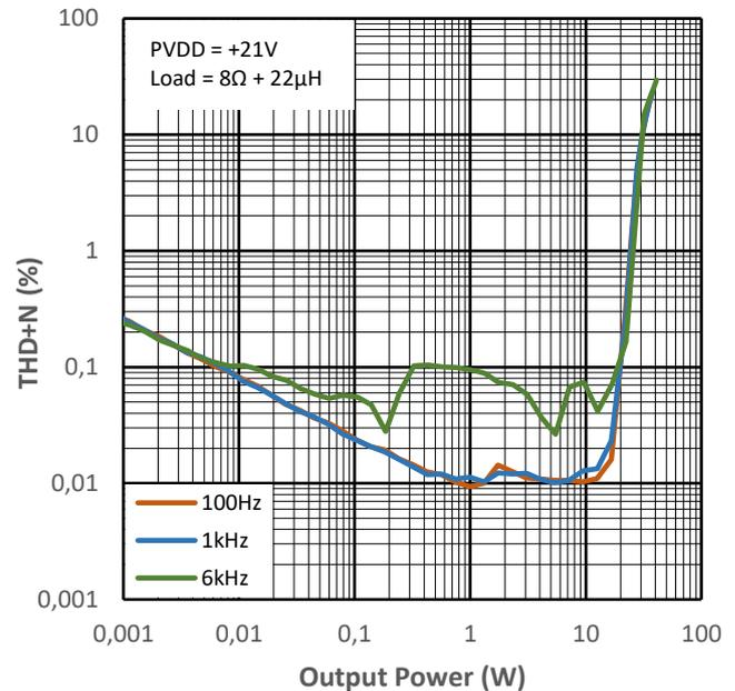
Figure 15-4 THD+N vs Output Power for PMP4
