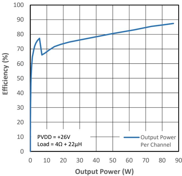
Figure 10-11 PMP2 Efficiency (VDD+PVDD) vs Output Power
