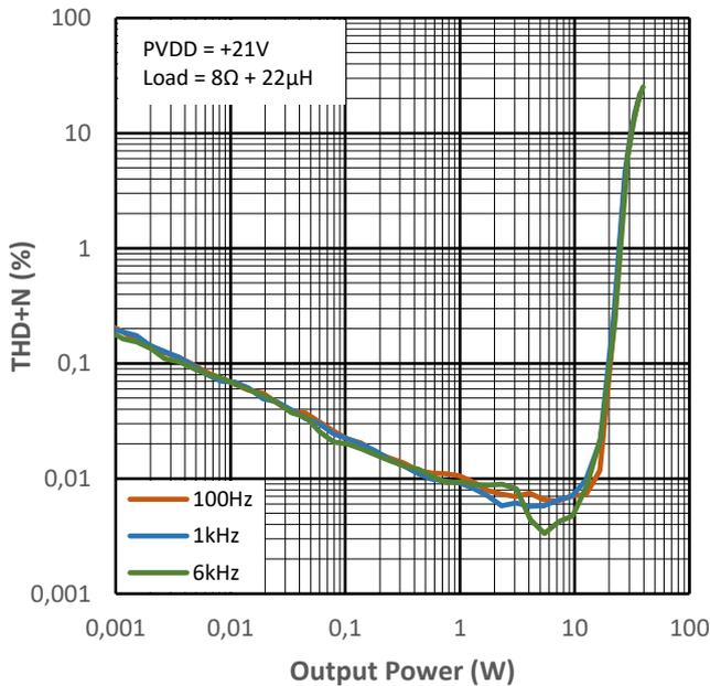
Figure 15-3 THD+N vs Output Power for PMP2
