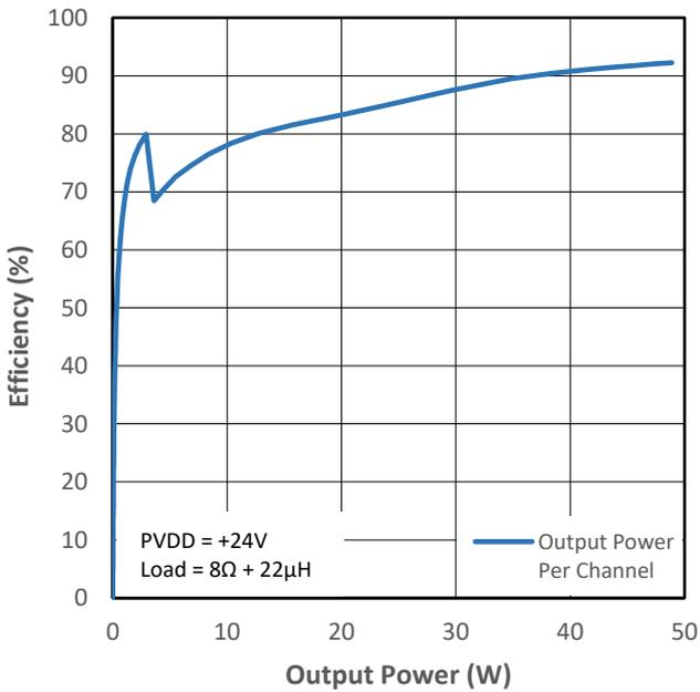
Figure 13-11 PMP2 Efficiency (VDD+PVDD) vs Output Power
