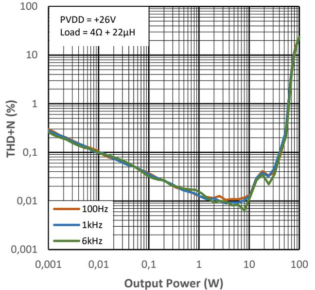
Figure 10-2 THD+N vs Output Power for PMP1
