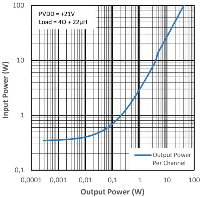
Figure 14-15 Input Power vs Output Power for PMP2
