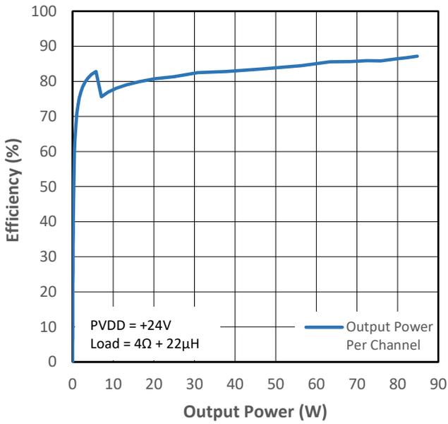
Figure 12-9 PMP0 Efficiency (VDD+PVDD) vs Output Power
