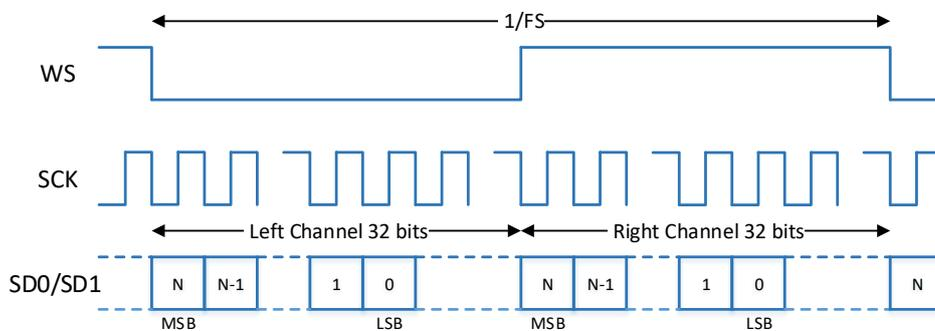
**Figure 8-2 Timing diagram of left justified mode (default).**
