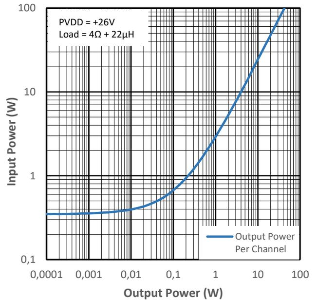
Figure 10-16 Input Power vs Output Power for PMP4
