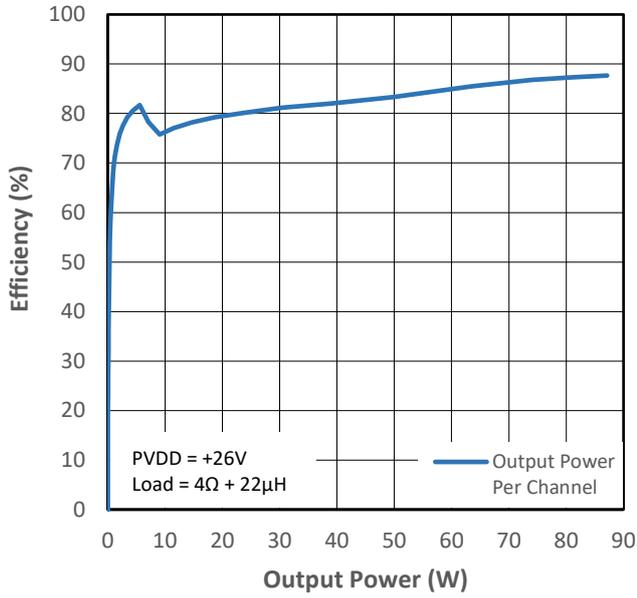
Figure 10-9 PMP0 Efficiency (VDD+PVDD) vs Output Power
