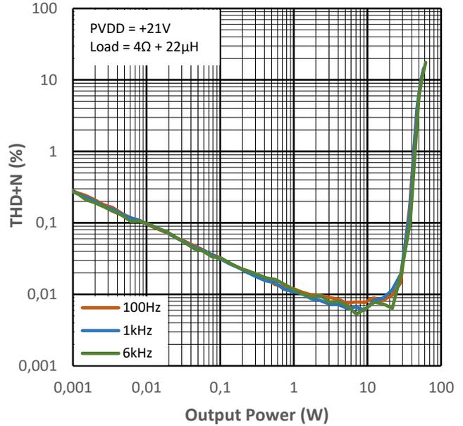
Figure 14-2 THD+N vs Output Power for PMP1
