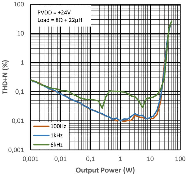
Figure 13-1 THD+N vs Output Power for PMP0
