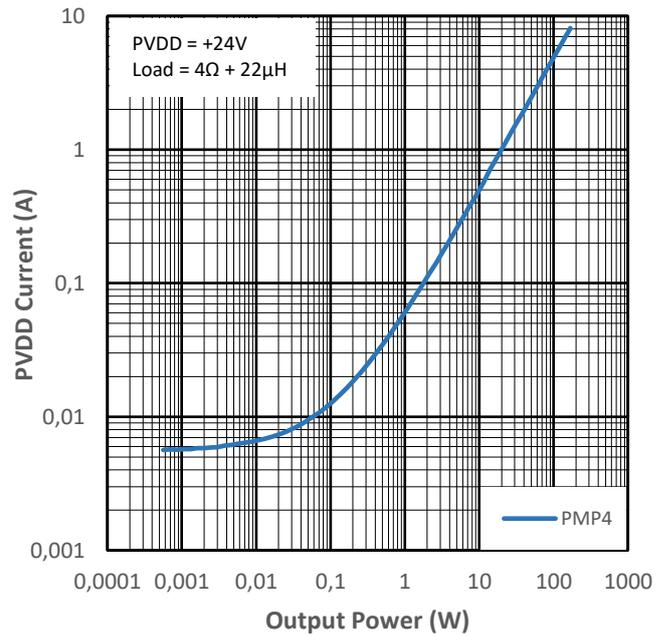
Figure 12-20 PVDD Current vs Output Power for PMP4
