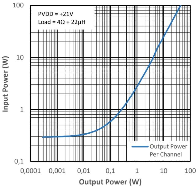
Figure 14-13 Input Power vs Output Power for PMP0
