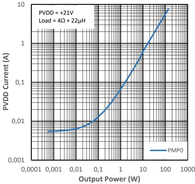
Figure 14-17 PVDD Current vs Output Power for PMP0
