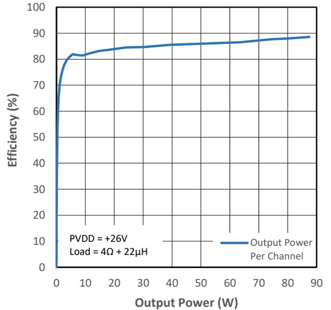
Figure 10-12 PMP4 Efficiency (VDD+PVDD) vs Output Power
