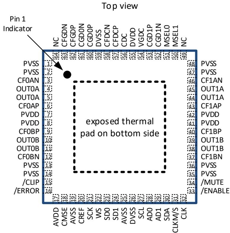
Figure 4-1 Pinout MA12070P
