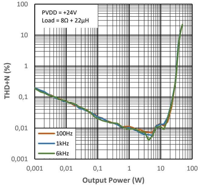
Figure 13-2 THD+N vs Output Power for PMP1
