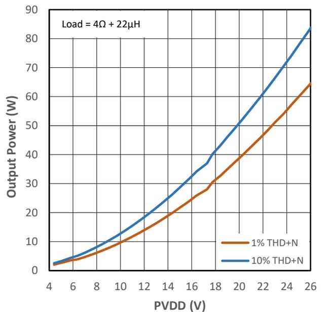
Figure 10-24 Output Power vs PVDD for PMP4
