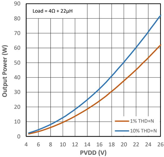
Figure 10-21 Output Power vs PVDD for PMP0
