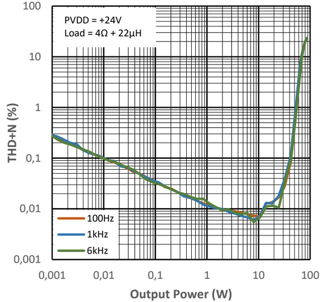
Figure 12-2 THD+N vs Output Power for PMP1
