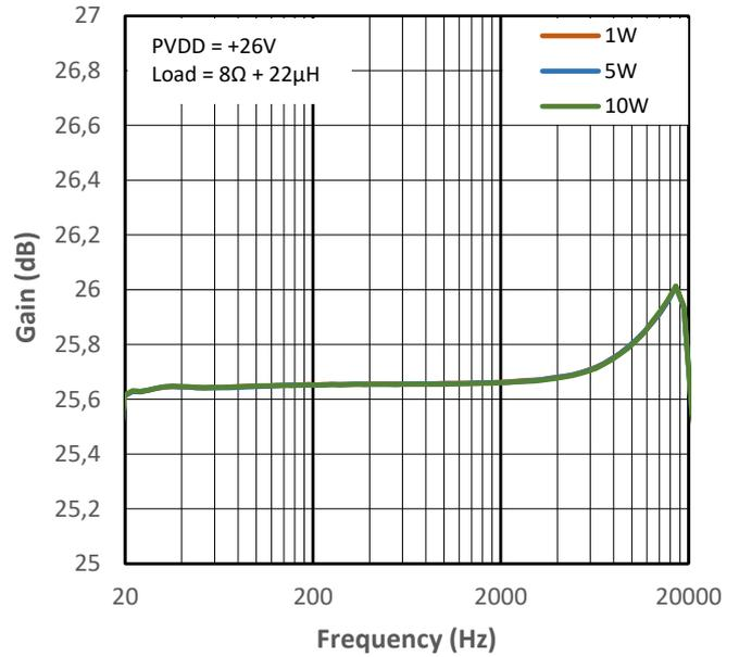
Figure 11-26 Gain vs Frequency for PMP1
