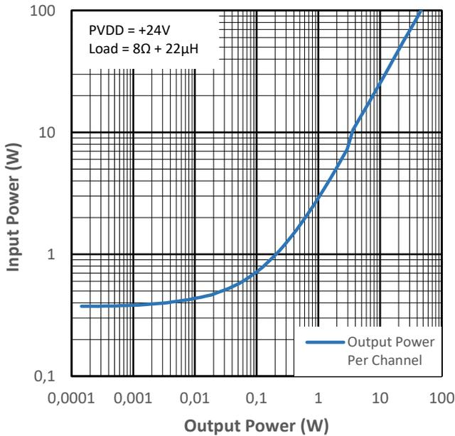
**Figure 13-15 Input Power vs Output Power for PMP2**
