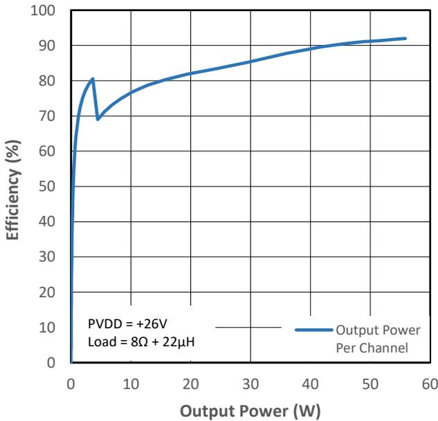
Figure 11-11 PMP2 Efficiency (VDD+PVDD) vs Output Power
