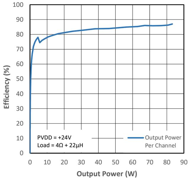
Figure 12-10 PMP1 Efficiency (VDD+PVDD) vs Output Power
