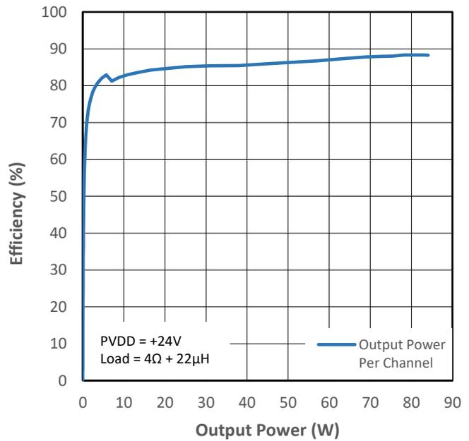
Figure 12-12 PMP4 Efficiency (VDD+PVDD) vs Output Power
