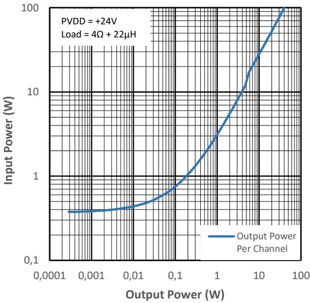
Figure 12-15 Input Power vs Output Power for PMP2
