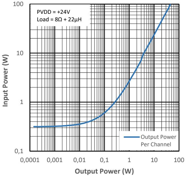
**Figure 13-13 Input Power vs Output Power for PMP0**
