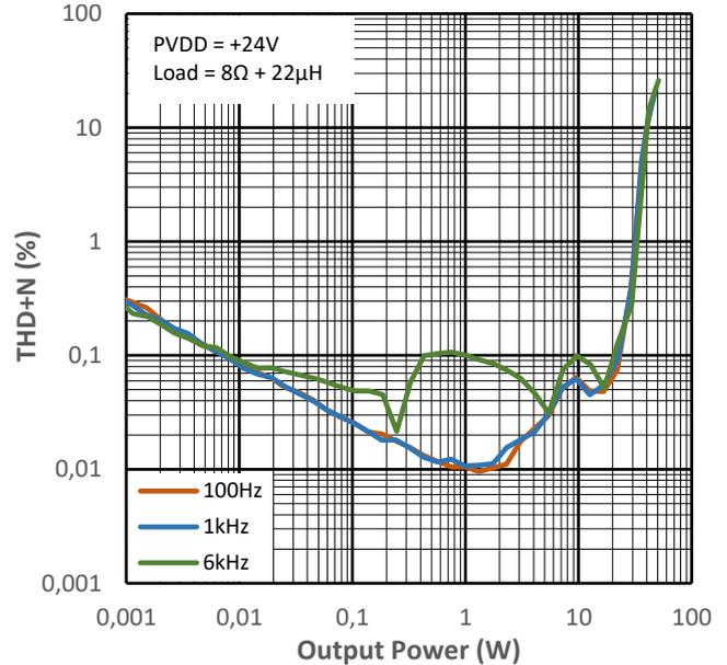
Figure 13-4 THD+N vs Output Power for PMP4
