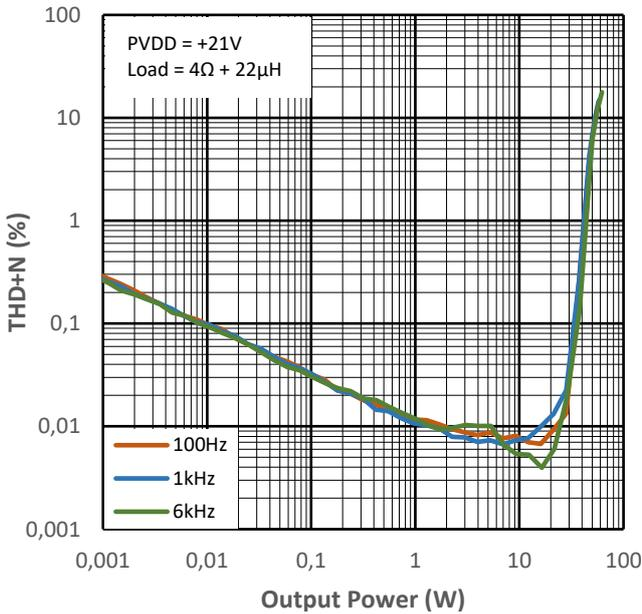
Figure 14-3 THD+N vs Output Power for PMP2
