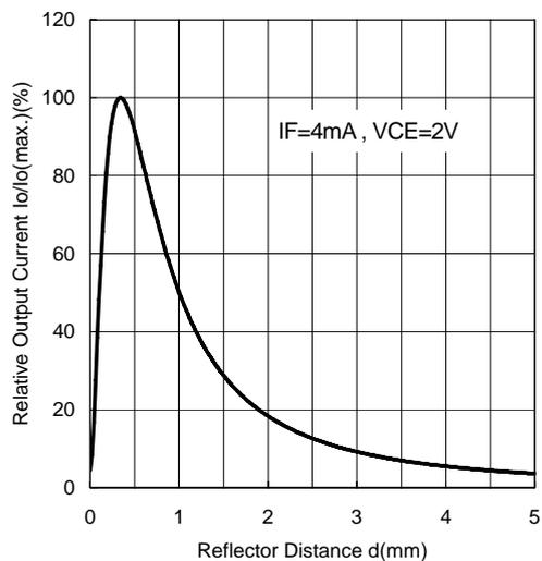
**Output Current vs. Edge Distance** ( $T_a=25^\circ\text{C}$ )
