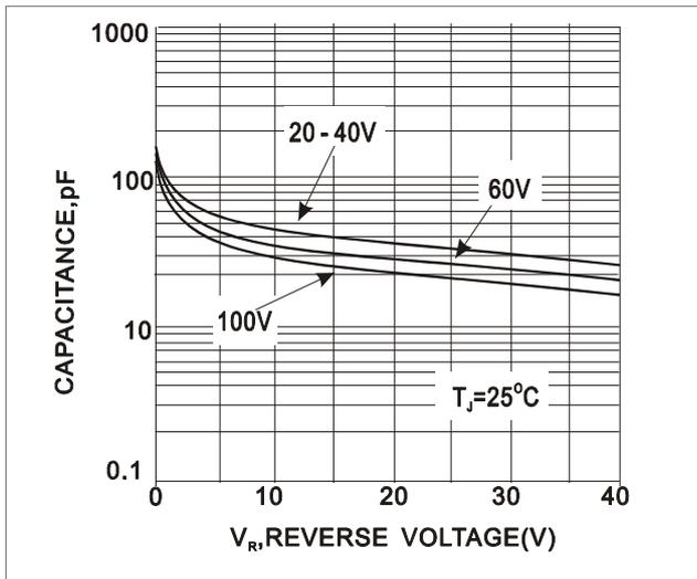
FIG. 3 TYPICAL JUNCTION CHARACTERISTIC
