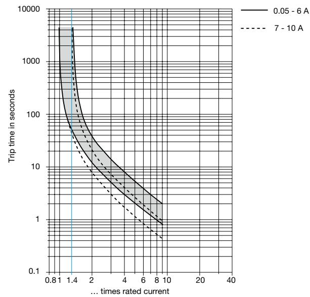
The time/current characteristic depends on the ambient temperature. In order to eliminate nuisance tripping, please multiply the current rating with a temperature factor (see Technical Information chapter)
