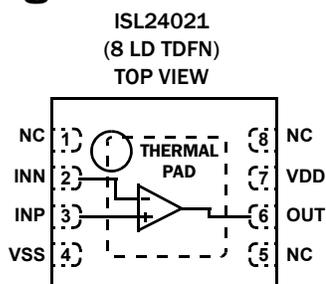
THERMAL PAD IS ELECTRICALLY ISOLATED, OR CONNECTED TO VSS
