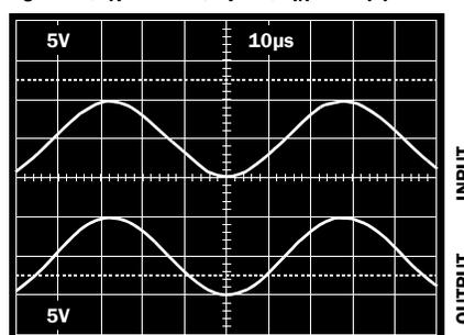
FIGURE 24. OPERATION WITH RAIL-TO-RAIL INPUT AND OUTPUT
