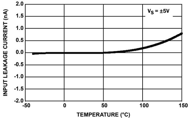
FIGURE 3. INPUT LEAKAGE CURRENT vs TEMPERATURE
