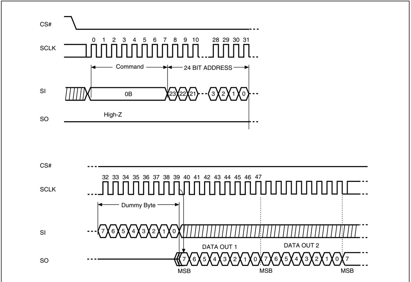
**Figure 18. Dual Output Read Mode Sequence (Command 3B)**
