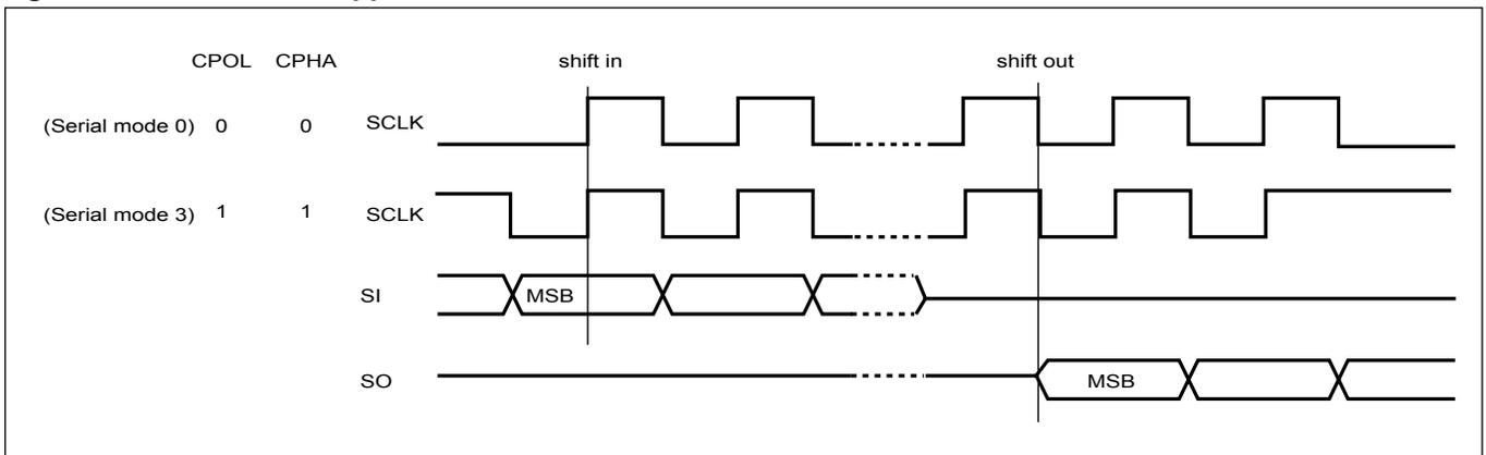
**Note:** CPOL indicates clock polarity of Serial master:
