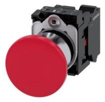
Mushroom pushbutton, 22 mm, round, metal, shiny, red, 40mm, latching, pull-to-unlatch mechanism, with holder, 1 NC, spring-type terminal, Z=20-unit packaging
