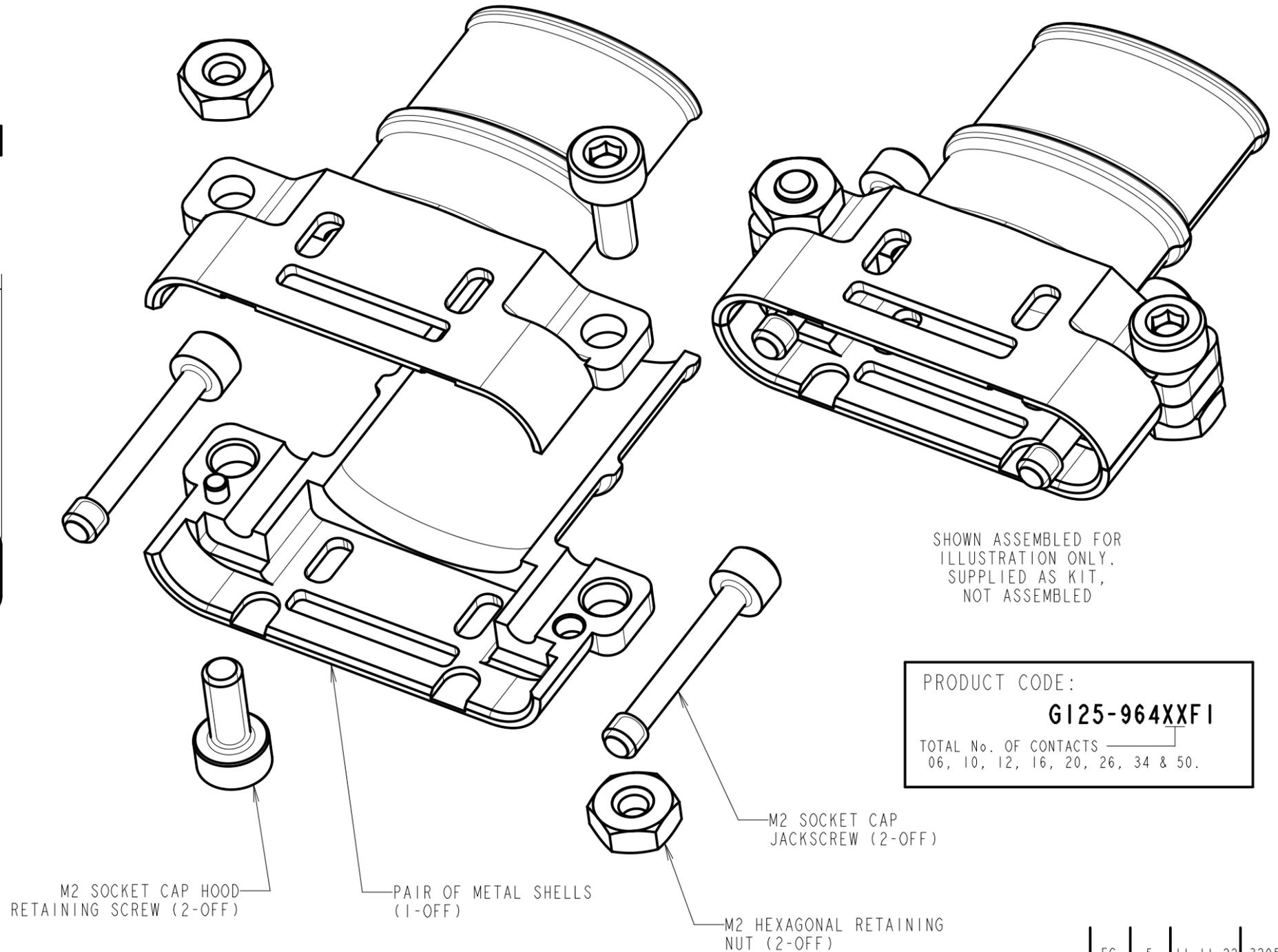
SHOWN ASSEMBLED FOR ILLUSTRATION ONLY. SUPPLIED AS KIT, NOT ASSEMBLED
