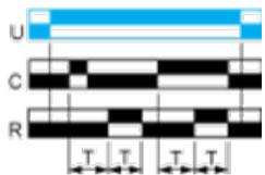
Function N : Retriggerable Interval Relay with Control Signal On
