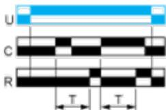
Function Ah : Pulse Delayed Relay (Single Cycle) with Control Signal
