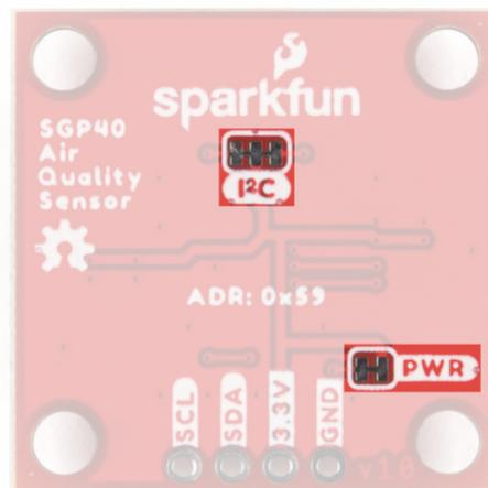
Disable the Power LED by severing the trace between the two pads. Opening this jumper helps reduce the total current draw of the breakout for low-power applications. Similarly, disable the pull-up resistors for the SDA/SCL lines by severing the trace between the three pads.
