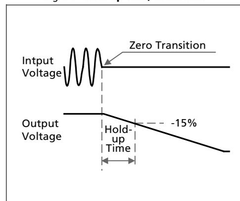
Fig. 8-2 **Hold-up time vs. input voltage**
