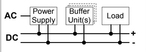
Do not use the buffer module to bridge mains interruptions which are longer than typ. 350ms. Once the mains is off for longer than typ. 350ms, the XT power supply needs an additional 1s to restart again.
