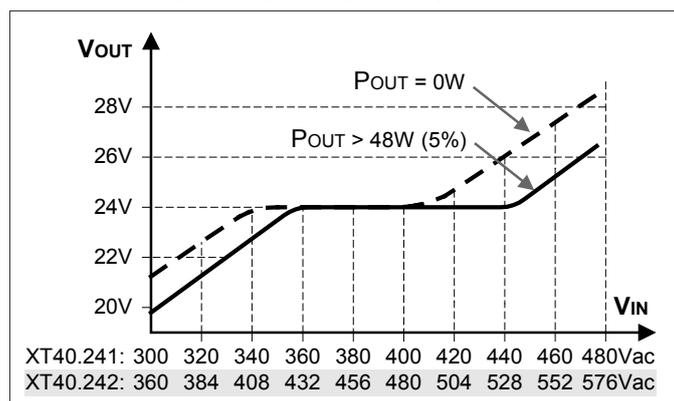
Fig. 5-2 **Input voltage range**
