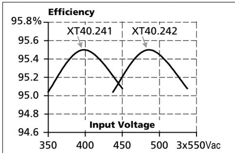
Fig. 9-4 Losses vs. input voltage, 24V, 40A
