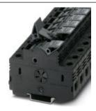
Fuse modular terminal block, Connection method: Screw connection, Cross section: 1.5 mm²- 25 mm², AWG: 16 - 4, Nominal current: 32 A, Nominal voltage: 690 V, Width: 18 mm, Fuse type: Midget / 10.3 x 38, Fuse type: Glass, Mounting type: NS 35/7,5, NS 35/15, Color: black
