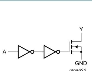
**Fig. 3. Logic diagram (one inverter)**
