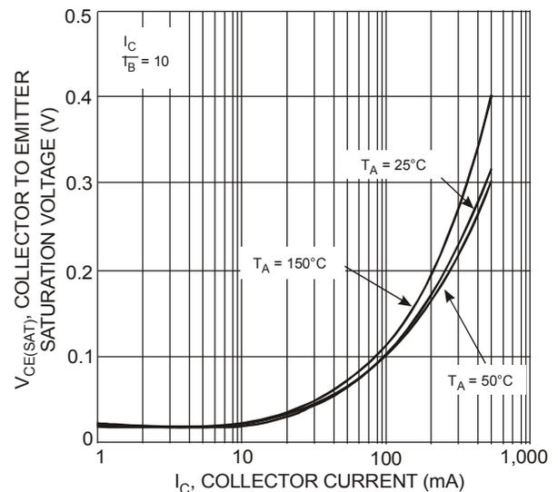
Fig. 2 Collector Emitter Saturation Voltage vs. Collector Current
