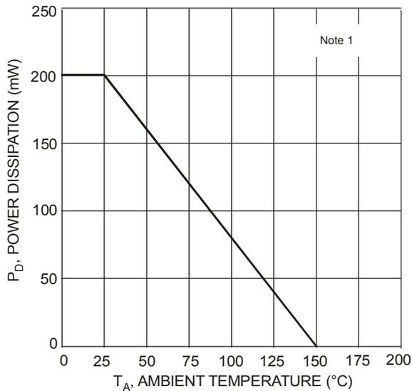
Fig. 1 Max Power Dissipation vs. Ambient Temperature
