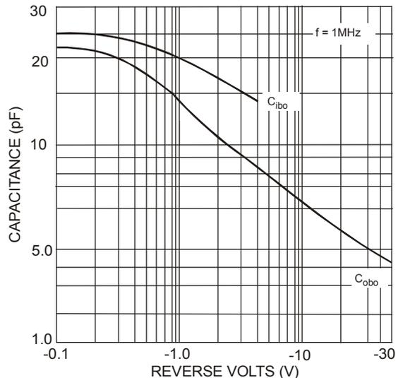
Fig. 6 Typical Capacitance
