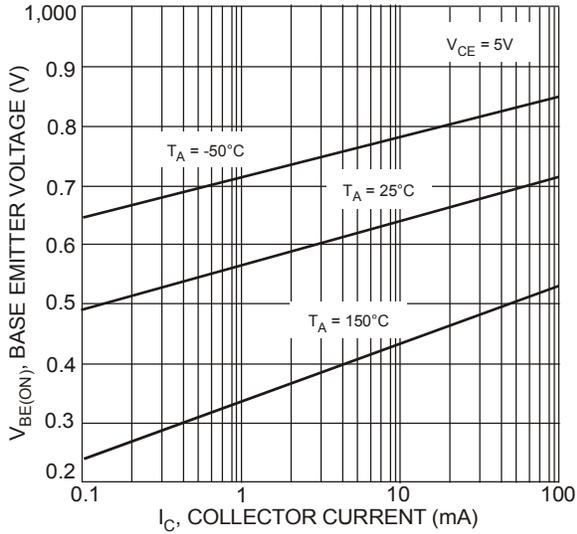
Fig. 3 Base-Emitter Voltage vs. Collector Current
