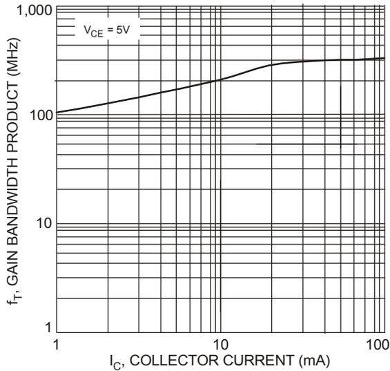
Fig. 5 Gain Bandwidth Product vs. Collector Current
