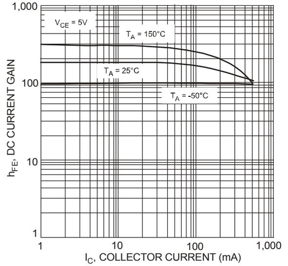
Fig. 4 DC Current Gain vs. Collector Current
