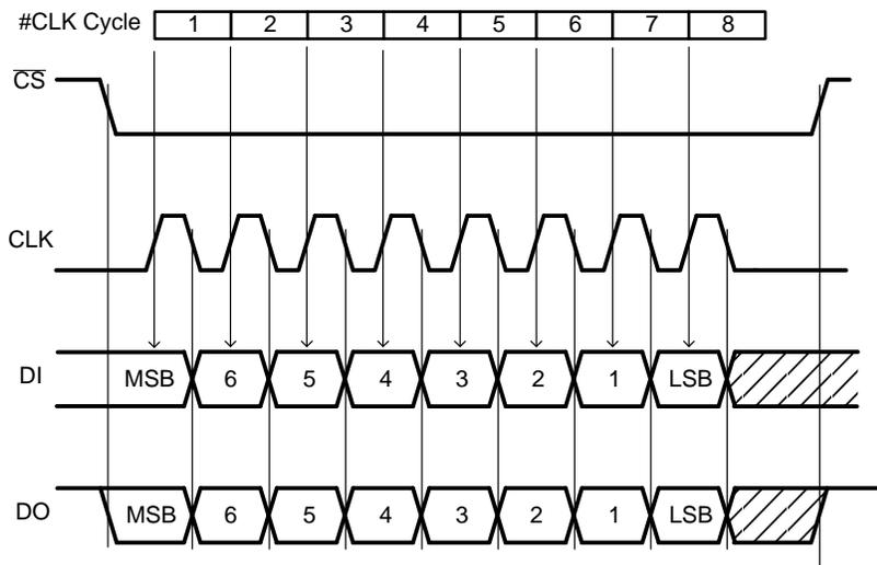
Figure 16. Timing Diagram of a SPI Transfer
