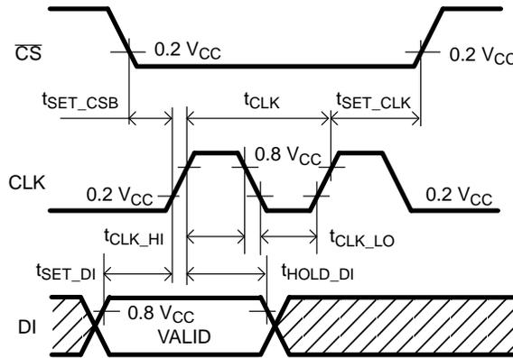
Figure 4. SPI Timing
