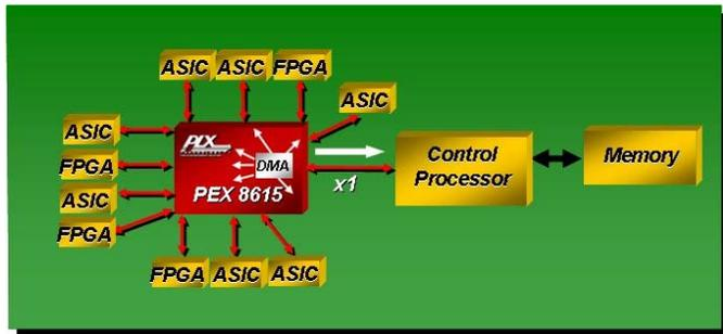
Figure 4. PEX8615 DMA in a Packet Router
