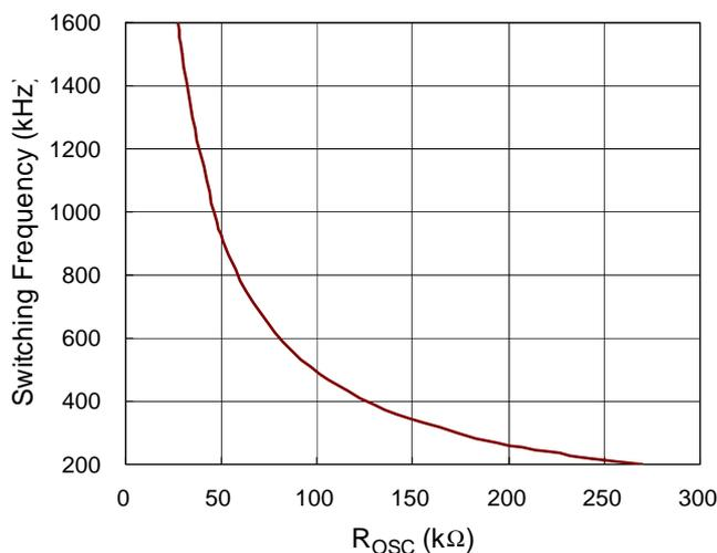
Figure 7. Switching Frequency vs. R<sub>osc</sub> Resistor
