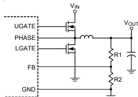
Figure 4. Setting V<sub>OUT</sub> with a Resistor Divider
