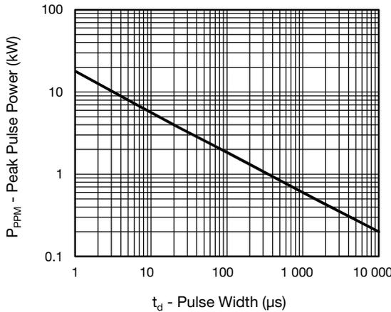
Fig. 1 - Peak Pulse Power Rating Curve
