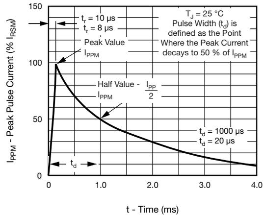
Fig. 3 - Pulse Waveform
