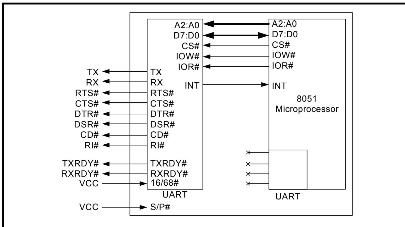
In the serial mode, the external serial port will need to communicate with the UART via AT commands.
