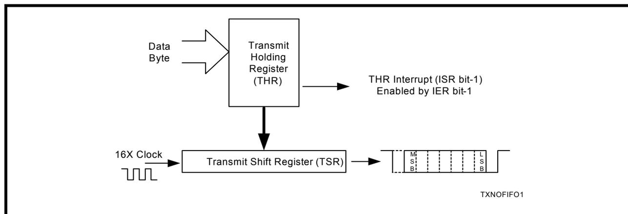
**3.9.3 Transmitter Operation in FIFO Mode**
