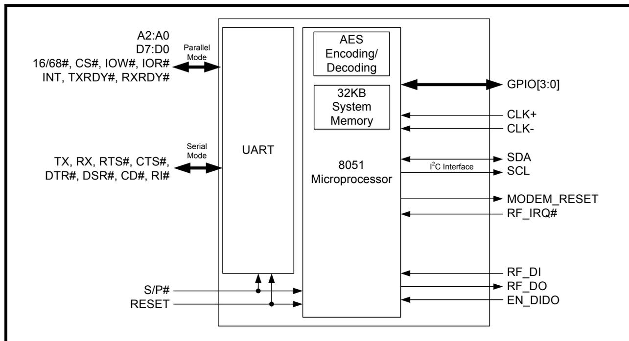
**FIGURE 2. PIN OUT ASSIGNMENT**
