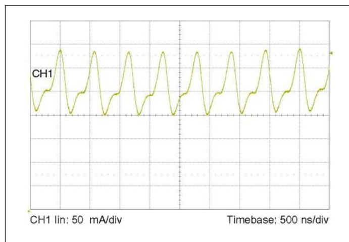
**Figure 4** — Input reflected ripple current at full load and 48 V<sub>IN</sub>
