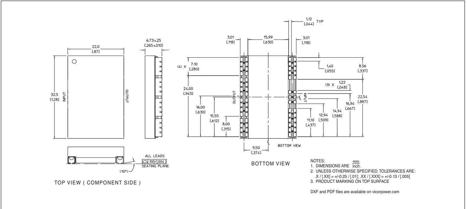
Figure 15 — BCM® module J-Lead mechanical outline; onboard mounting
