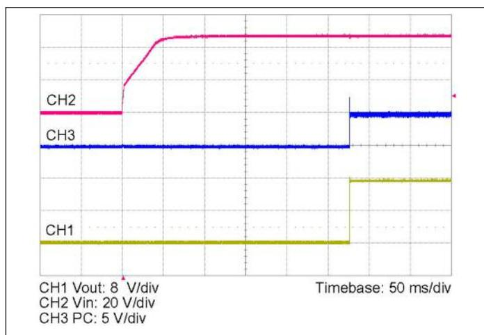
**Figure 3** — Output voltage turn on waveform with input turn on at full load and 48 V<sub>IN</sub>
