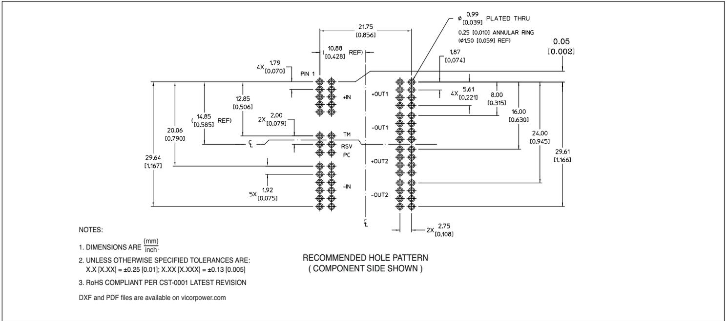
Figure 18 — BCM through-hole module PCB layout information
