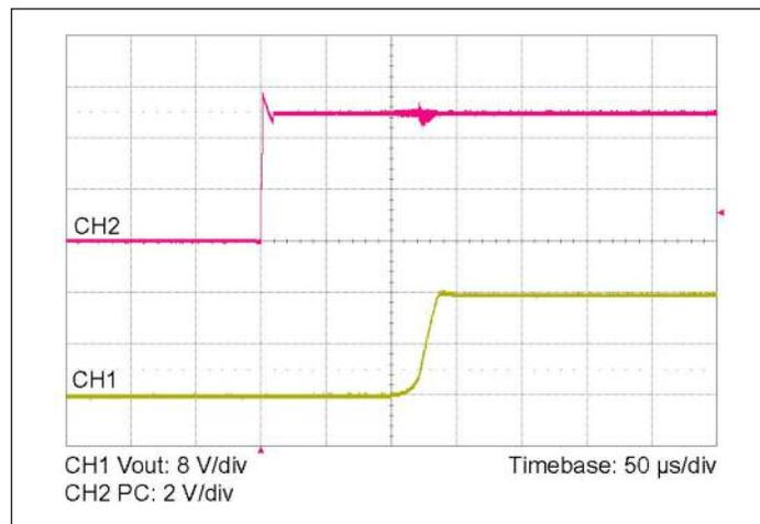
**Figure 2** — Output voltage turn on waveform with PC enabled at full load and 48 V<sub>IN</sub>
