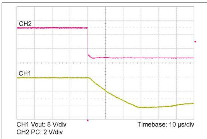
Figure 12 —  $V_{OUT}$  at full load vs. PC disable
