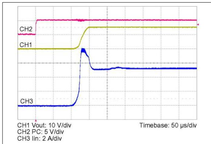
**Figure 1** — Inrush transient current at full load and 48 V<sub>IN</sub> with PC enabled
