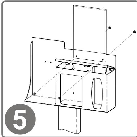
To mount the MP-070 Sign Holder, align the mounting holes of the holder with the holes on the top front of the dispenser. Attach using (2x) barrel screws included with sign holder.
