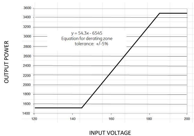
Figure 18. Output power derating below  $V_{IN}$  of 185V<sub>AC</sub>
