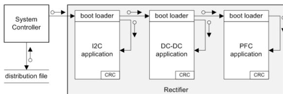
Each of the μControllers contains a **boot loader** section and an **application** section in memory. The purpose of the boot loader section is to facilitate the upgrading capability described here. All the commands for upgrading and memory space required for incrementally changing the application code are in this section. The application section contains the running code of the rectifier.
