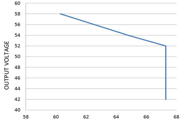
Figure 4. 54V<sub>DC</sub> output: Power limit, Current limit and shutdown profile at  $V_{IN} = 185V_{AC}$ .
