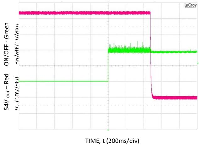
Figure 16. 54V<sub>DC</sub> turn-OFF delay when ON/OFF is di-asserted,  $V_{IN}=230V_{AC}$  - I<sup>2</sup>C mode.
