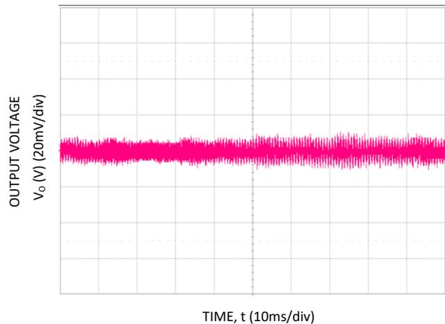
Figure 6. 5V<sub>DC</sub> output ripple and noise, all full load,  $V_{IN} = 185V_{AC}$ , 20MHz bandwidth
