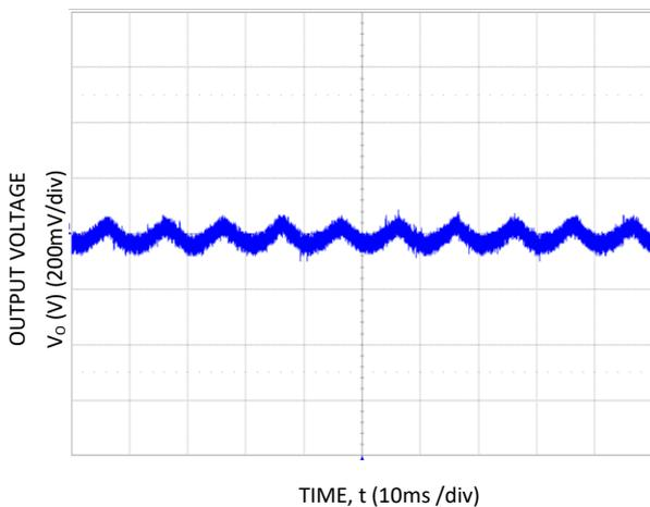
Figure 5. 54V<sub>DC</sub> output ripple and noise, full load,  $V_{IN} = 185V_{AC}$ , 20MHz bandwidth
