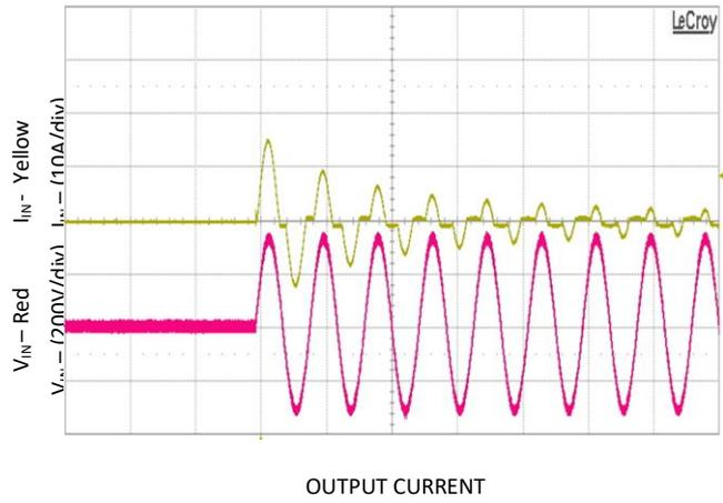
Figure 2. Inrush current  $V_{IN} = 230V_{AC}$ , 0° phase angle
