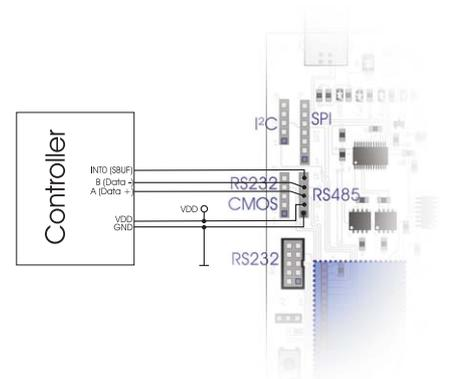
**DIP-Switch setting: RS232, RS485, RS232 CMOS (EA 9777-2PE)**
