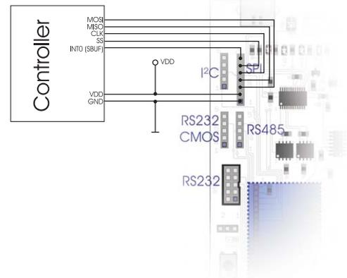
**DIP-Switch setting: SPI-Interface (EA 9777-2PE)**
