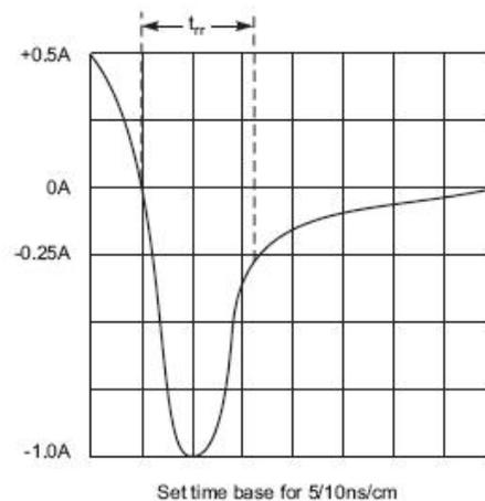
Fig. 5 Reverse Recovery Time Characteristic and Test Circuit
