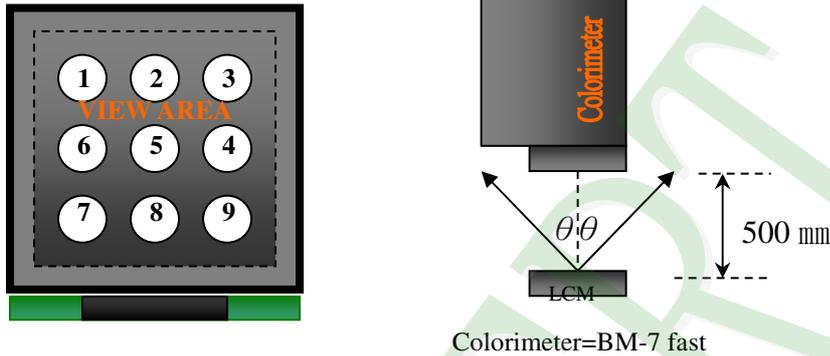
To be measured at the center area of panel with a viewing cone of  $1^{\circ}$  by Topcon luminance meter BM-7, after 10 minutes operation (module)
