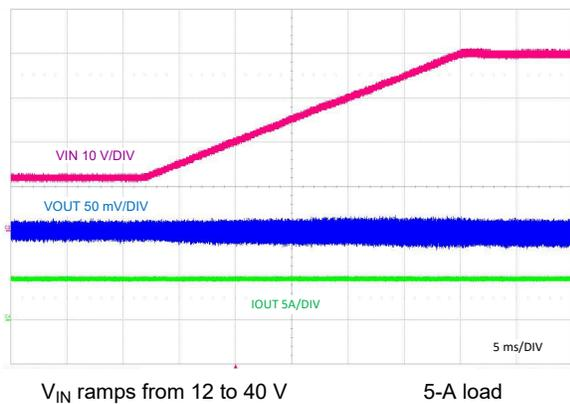
Figure 9-23. Line Transient Response to  $V_{IN} = 40\text{ V}$
