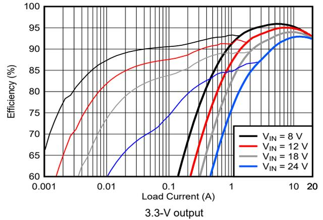
**Figure 9-31. Efficiency vs.  $I_{OUT}$ , Log Scale**
