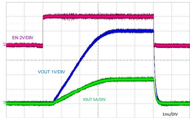
V<sub>IN</sub> = 12 V 8-A resistive load
