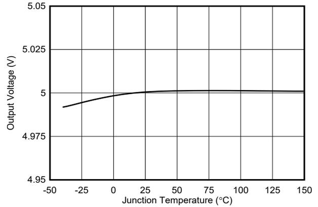
**Figure 7-8. Fixed 5-V Output Voltage vs. Temperature**
