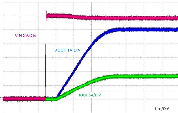
V<sub>IN</sub> step to 12 V 8-A resistive load
