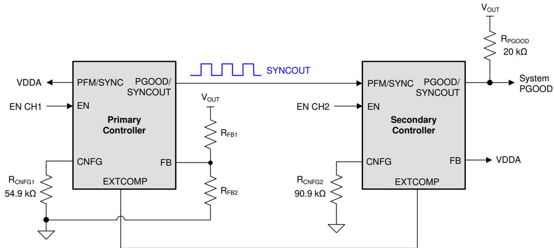
**Figure 8-7. Schematic Configured for Single-Output Dual-Phase Operation**
