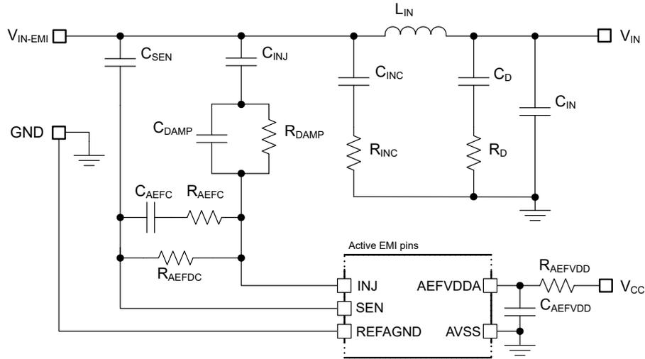
Figure 9-3. Active EMI Filter for a Buck Regulator
