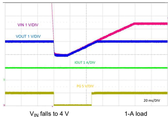
Figure 9-24. Line Transient Response to  $V_{IN} = 4\text{ V}$
