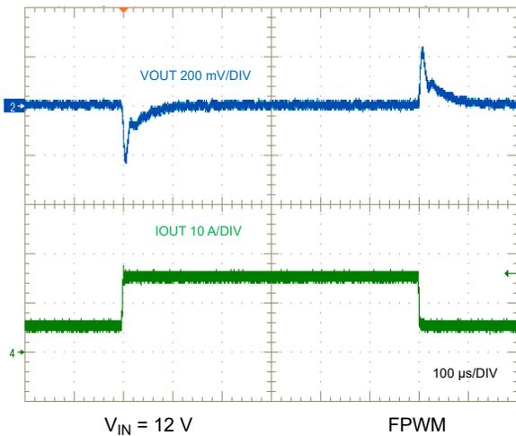
**Figure 9-34. Load Transient, 5 A to 15 A**
