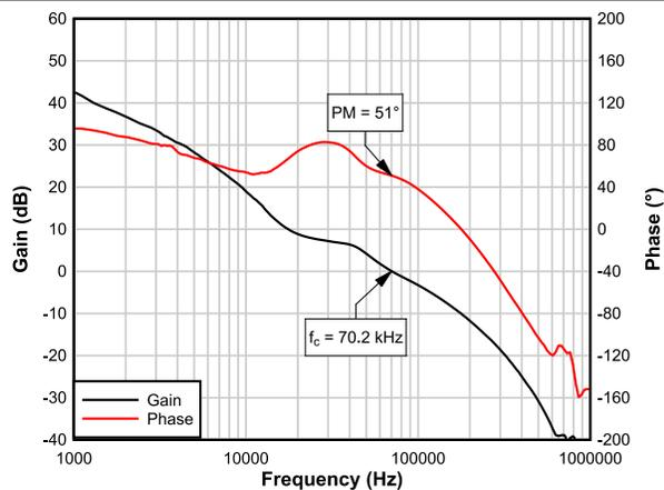
V<sub>IN</sub> = 12 V 8-A resistive load
