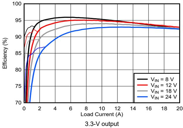
**Figure 9-30. Efficiency vs.  $I_{OUT}$**
