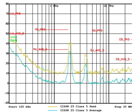
V<sub>IN</sub> = 13.8 V 150 kHz to 30 MHz 7-A resistive load
