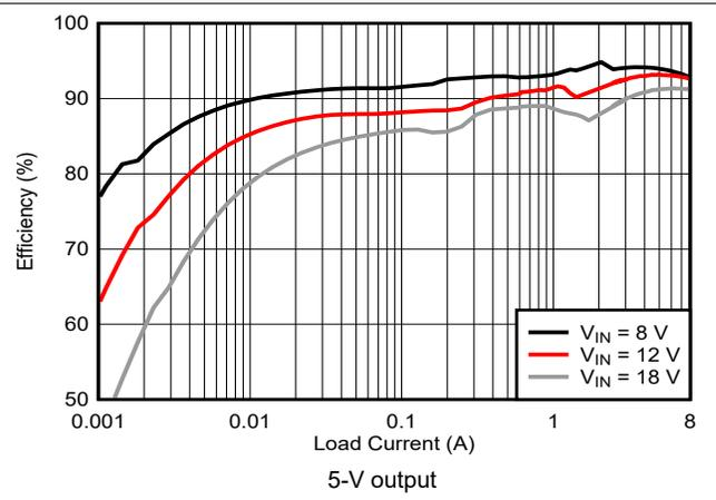
**Figure 9-7. Efficiency vs.  $I_{OUT}$ , Log Scale**
