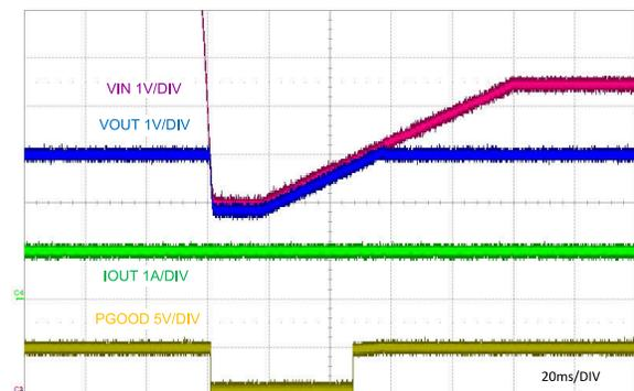
**Figure 9-11. Line Transient Response to  $V_{IN} = 4$  V**
