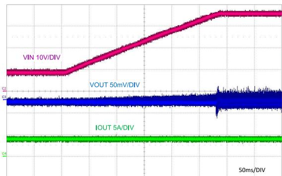
**Figure 9-10. Line Transient Response to  $V_{IN} = 36$  V**
