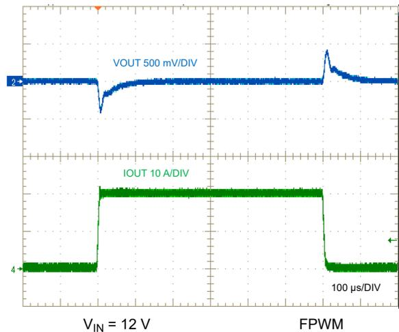
**Figure 9-35. Load Transient, 0 A to 20 A**
