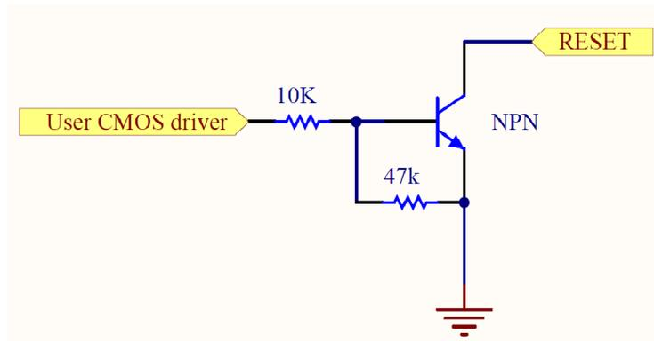
Figure 5 Reset Pin Diagram
