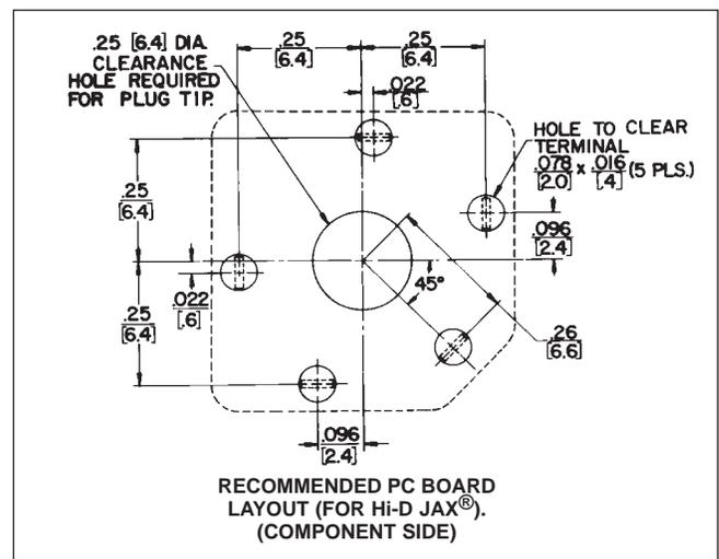
DIMENSIONS ARE FOR REFERENCE ONLY  $\frac{\text{Inch}}{\text{mm}}$
