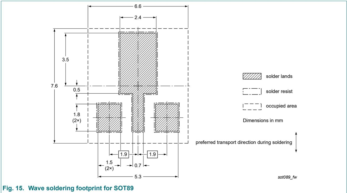
Fig. 15. Wave soldering footprint for SOT89
