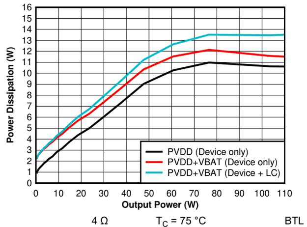
Figure 7-8. Power Dissipation vs Output Power - 14.4 V - 4  $\Omega$
