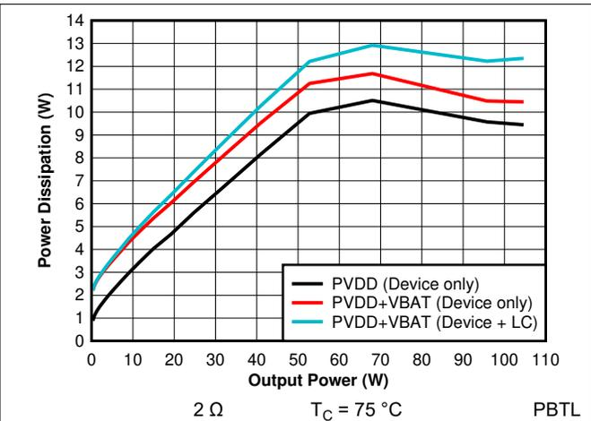
Figure 7-35. Power Dissipation vs Output Power - PBTL - 2  $\Omega$
