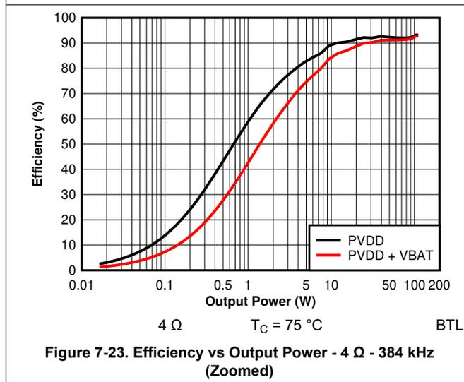
Figure 7-23. Efficiency vs Output Power - 4  $\Omega$  - 384 kHz (Zoomed)
