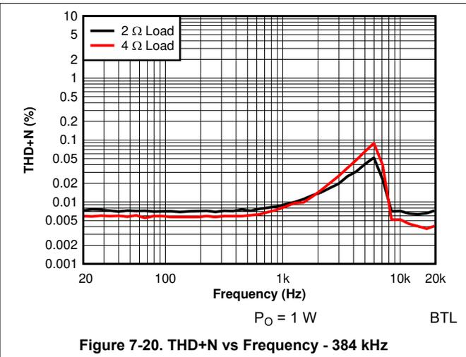
Figure 7-20. THD+N vs Frequency - 384 kHz
