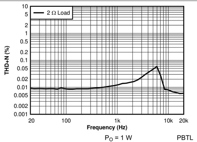
Figure 7-38. THD+N vs Frequency - PBTL - 384 kHz
