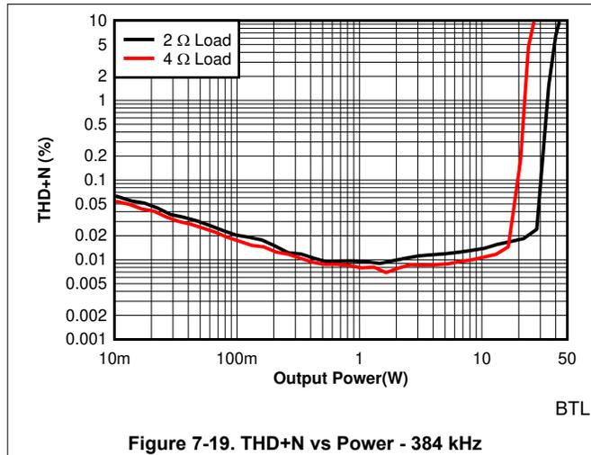
Figure 7-19. THD+N vs Power - 384 kHz
