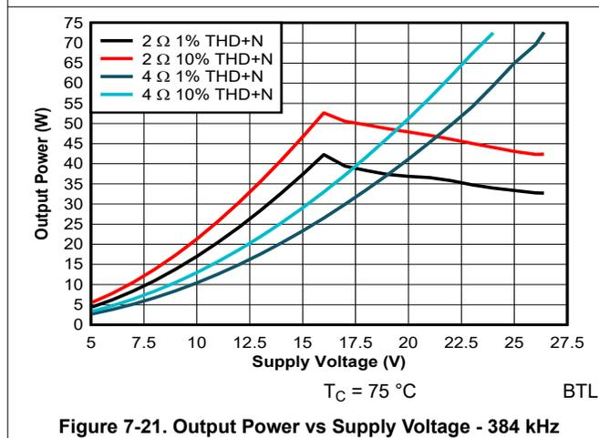
Figure 7-21. Output Power vs Supply Voltage - 384 kHz
