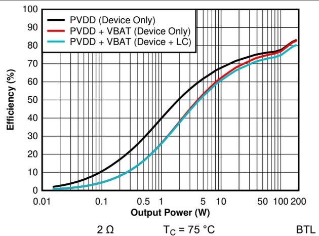
Figure 7-10. Efficiency vs Output Power - 14.4 V - 2  $\Omega$  (Zoomed)
