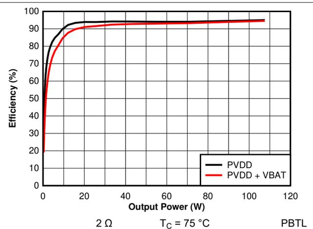
Figure 7-40. Efficiency vs Output Power - PBTL - 2  $\Omega$  - 384 kHz
