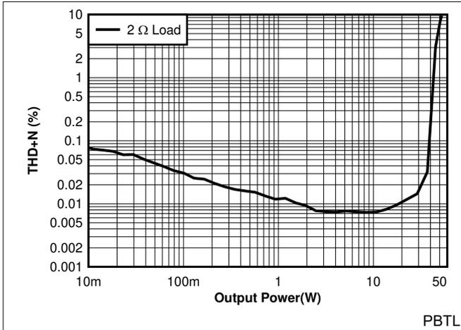
Figure 7-37. THD+N vs Power - PBTL - 384kHz
