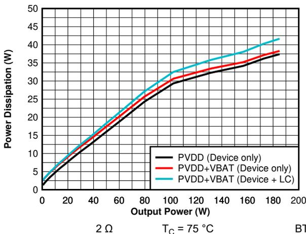
Figure 7-11. Power Dissipation vs Output Power - 14.4 V - 2  $\Omega$
