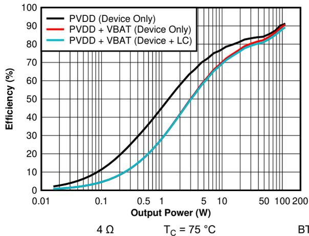
Figure 7-7. Efficiency vs Output Power - 14.4 V - 4  $\Omega$  (Zoomed)
