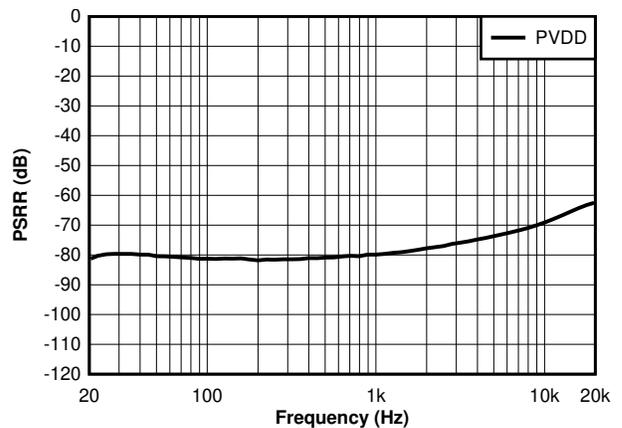
$P_O = 1\text{ W}$   $PVDD = 14.4\text{ V} + 1\text{ V}_{RMS}$  BTL
