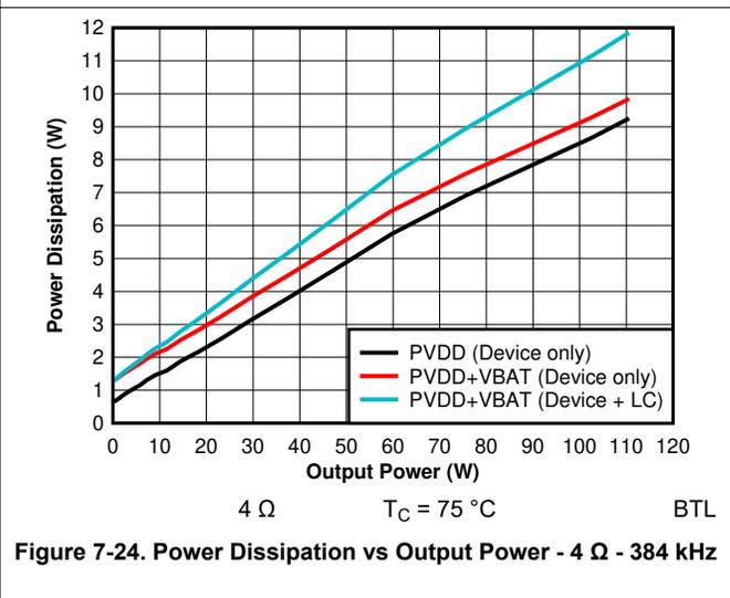
Figure 7-24. Power Dissipation vs Output Power - 4  $\Omega$  - 384 kHz
