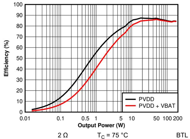
Figure 7-26. Efficiency vs Output Power - 2  $\Omega$  - 384 kHz (Zoomed)
