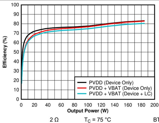
Figure 7-9. Efficiency vs Output Power - 14.4 V - 2  $\Omega$
