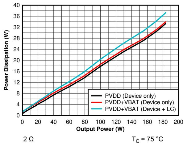
Figure 7-27. Power Dissipation vs Output Power - 2  $\Omega$  - 384 kHz
