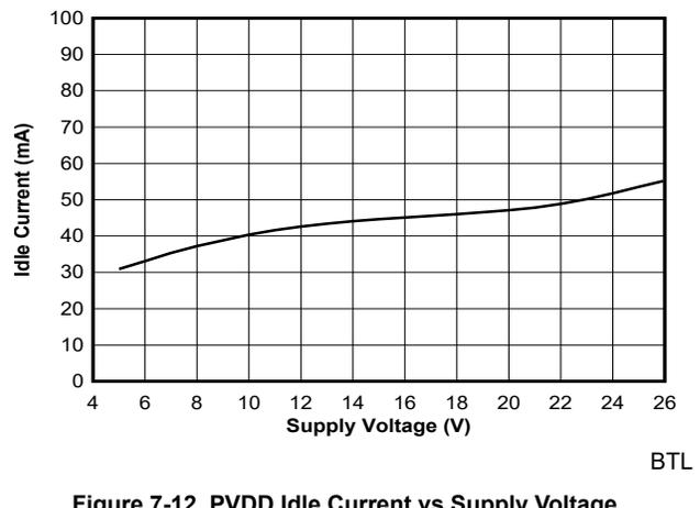
Figure 7-12. PVDD Idle Current vs Supply Voltage
