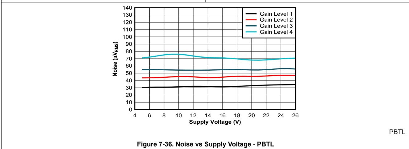
Figure 7-36. Noise vs Supply Voltage - PBTL
