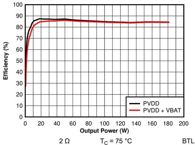
Figure 7-25. Efficiency vs Output Power - 2  $\Omega$  - 384 kHz
