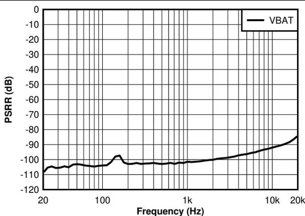
$P_O = 1\text{ W}$   $V_{BAT} = 14.4\text{ V} + 1\text{ V}_{RMS}$  BTL
