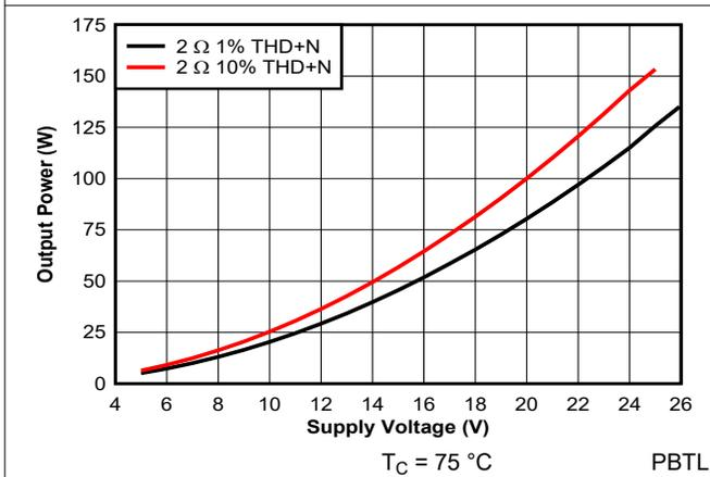
Figure 7-39. Output Power vs Supply Voltage - PBTL - 384 kHz
