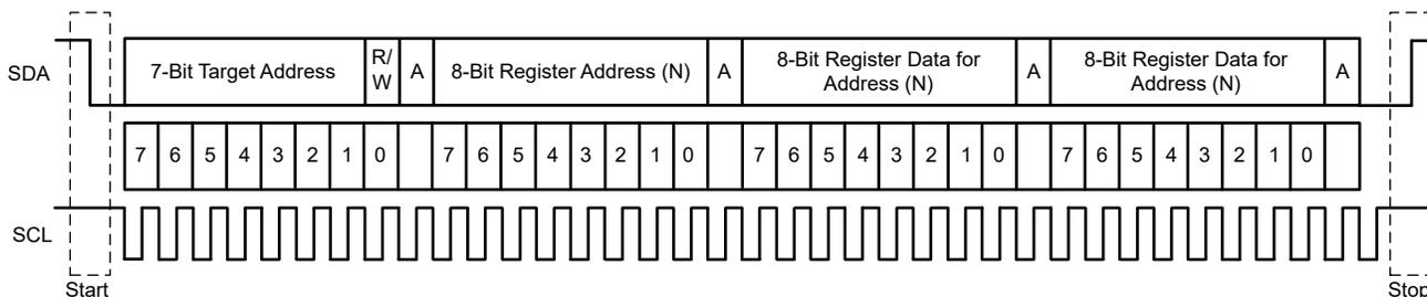
**Figure 9-8. Typical I<sup>2</sup>C Sequence**
