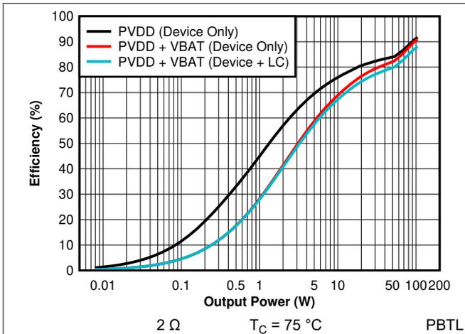
Figure 7-34. Efficiency vs Output power - PBTL - 2  $\Omega$  (Zoomed)
