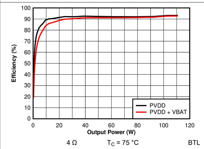
Figure 7-22. Efficiency vs Output Power - 4  $\Omega$  - 384 kHz
