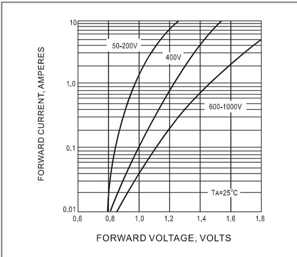
Fig.3 FORWARD CHARACTERISTICS
