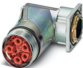
Device connector, front mounting, SB, angled rotatable, shielded: yes, for standard and SPEEDCON interlock, M40, No. of pos.: 4+4+4+PE, Direction of rotation: Standard, type of contact: Socket, Crimp connection, Axial O-ring, 4x Ø4,2, coding:CAT5, coding 1
