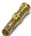
Crimp contact, turned, contact diameter: 1 mm, crimp range: 0.06 mm<sup>2</sup> ... 0.25 mm<sup>2</sup>
