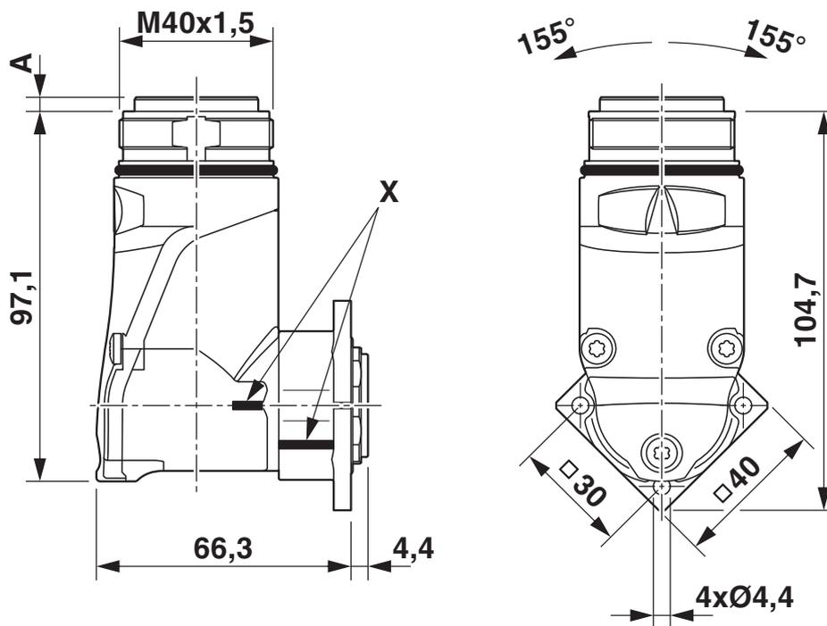
Pin version: dimension A = 3.7 mm, socket version: dimension A = 0.05 mm, X = reference position for angle of rotation
