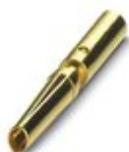
Crimp contact, turned, contact diameter: 0.8 mm, crimp range: 0.34 mm<sup>2</sup> ... 0.5 mm<sup>2</sup>
