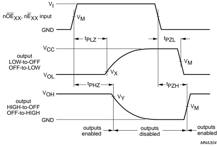
Fig.8 The 3-state enable and disable times.
