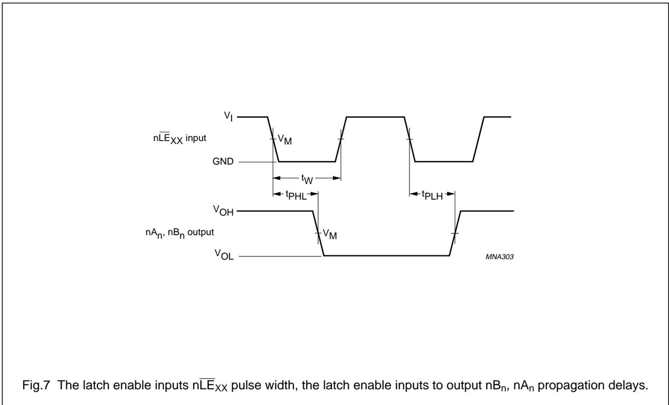
Fig.7 The latch enable inputs  $n\overline{LE}_{XX}$  pulse width, the latch enable inputs to output  $nB_n, nA_n$  propagation delays.
