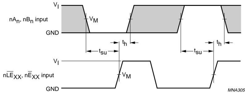
Fig.9 The data set-up and hold times for the  $nA_n, nB_n$  input to the  $n\overline{LE}_{XX}$  input.
