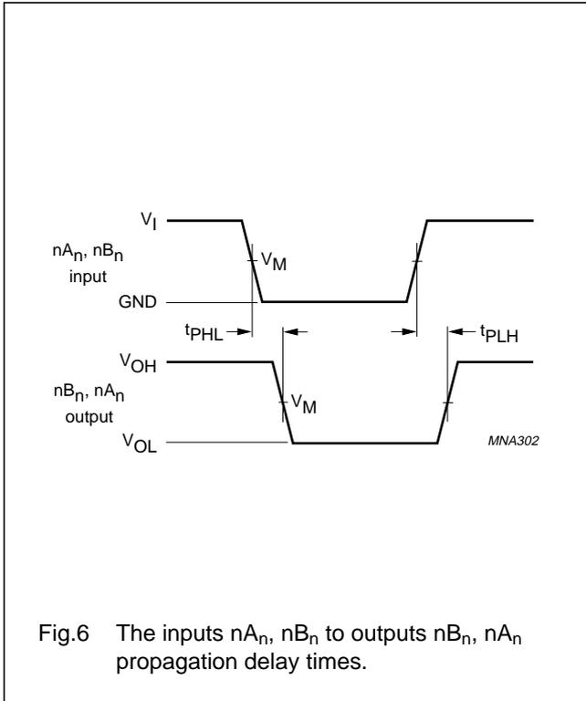
Fig.6 The inputs  $nA_n, nB_n$  to outputs  $nB_n, nA_n$  propagation delay times.
