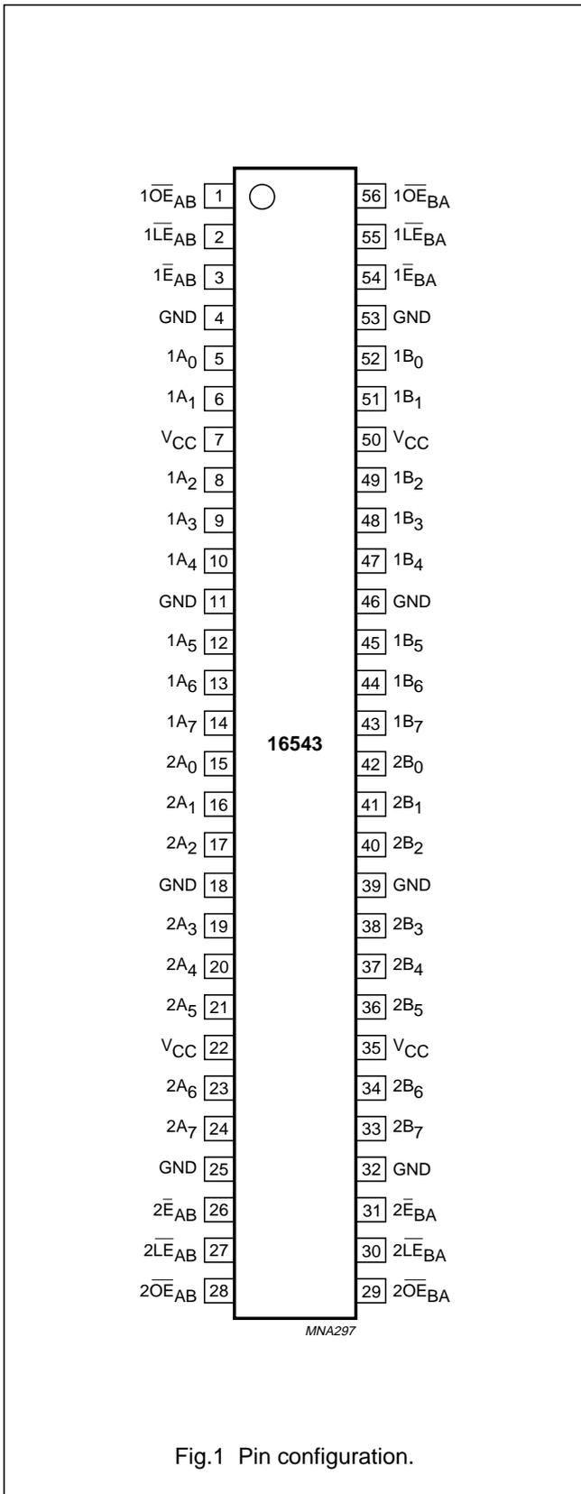
Fig.1 Pin configuration.
