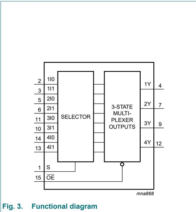
Fig. 3. Functional diagram
