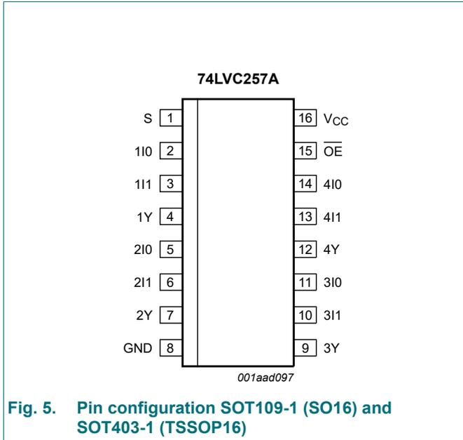
Fig. 5. Pin configuration SOT109-1 (SO16) and SOT403-1 (TSSOP16)
