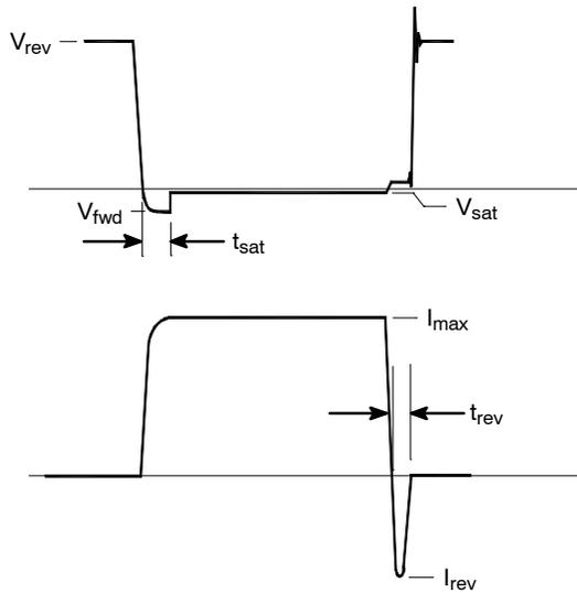
Figure 1. Switching Waveform
