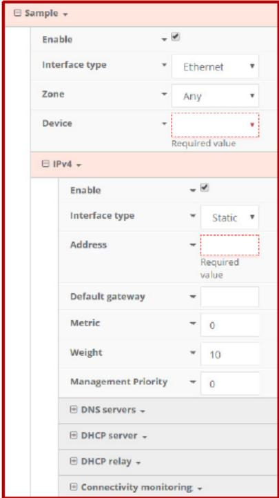
The screenshot shows the configuration page for a network interface. The 'Sample' interface is selected. The 'IPv4' section is expanded, showing the 'Address' field with a red dashed box around it, indicating it is a required value. Other fields like 'Default gateway', 'Metric', 'Weight', and 'Management Priority' are also visible.
