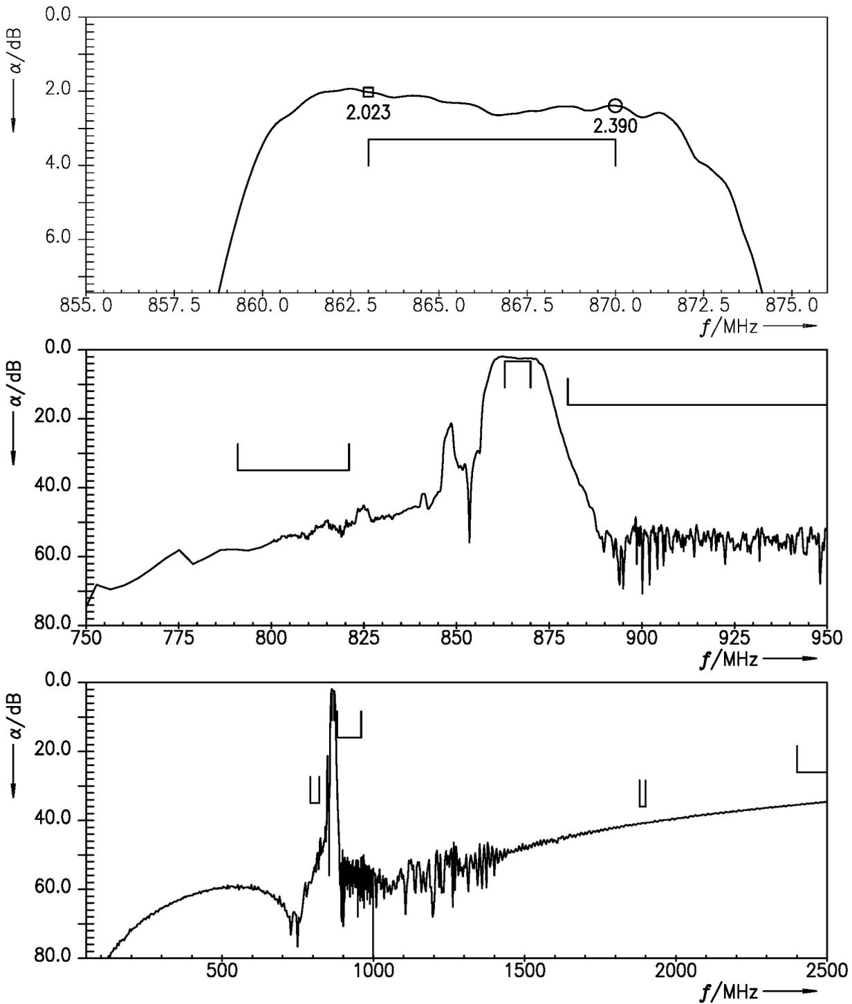
Figure 7: Attenuation Filter2.
