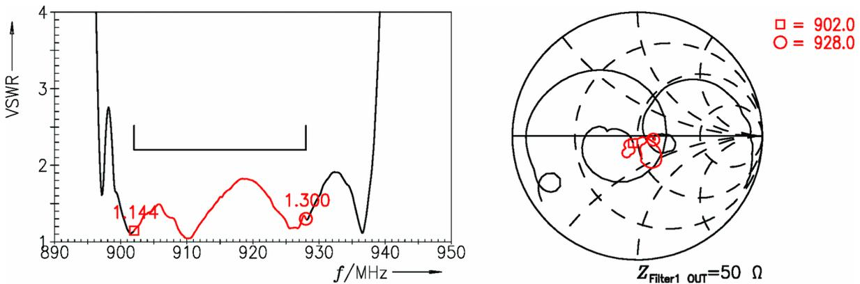
Figure 6: Reflection coefficient at Filter1 OUT port.
