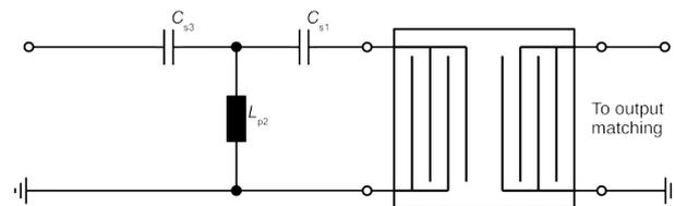
**Figure 17:** 3<sup>rd</sup> order high-pass structure for basic ESD protection.
