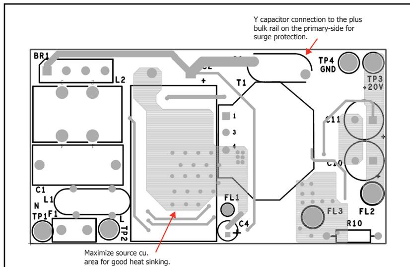
Figure 6. PCB Layout Top Side.
