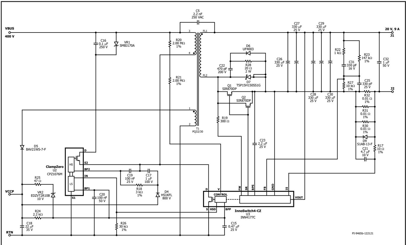
Figure 8. Schematic 20 V / 9 A Power Supply.
