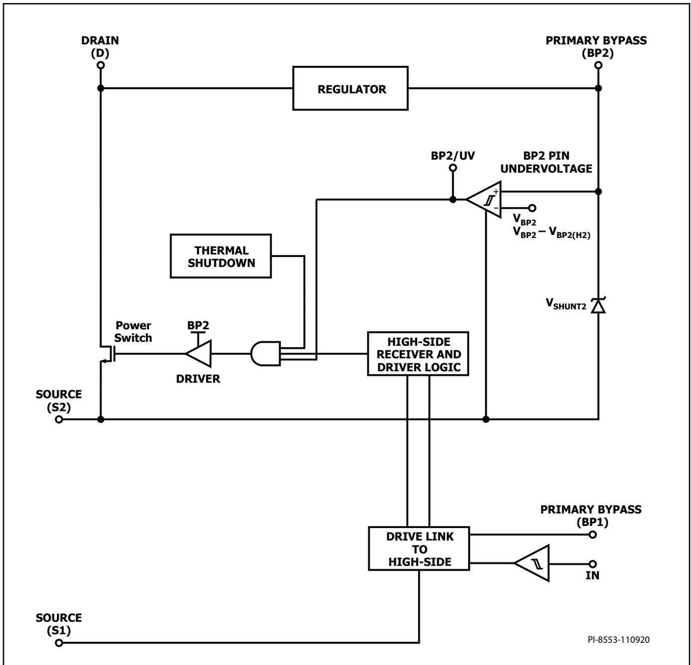
Figure 3. Block Diagram.
