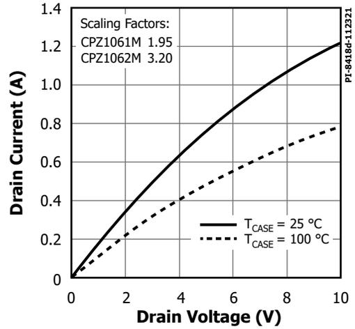
Figure 10. Output Characteristics.
