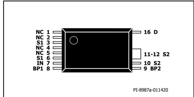
Figure 4. Pin Configuration.
