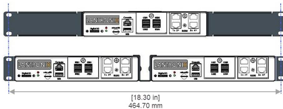
1. Attach the brackets on the sides of the EMG unit using a screwdriver and the screws provided with the mounting kit.
