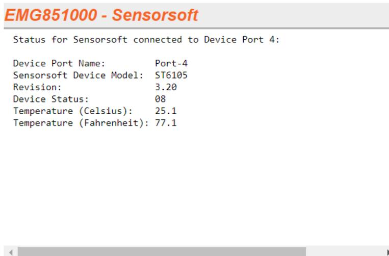
A screenshot of a web interface showing the status of a Sensorsoft device. The title is "EMG851000 - Sensorsoft". Below the title, it says "Status for Sensorsoft connected to Device Port 4:". A table-like list of key-value pairs follows: Device Port Name: Port-4, Sensorsoft Device Model: ST6105, Revision: 3.20, Device Status: 08, Temperature (Celsius): 25.1, and Temperature (Fahrenheit): 77.1. The interface has a scroll bar at the bottom.
