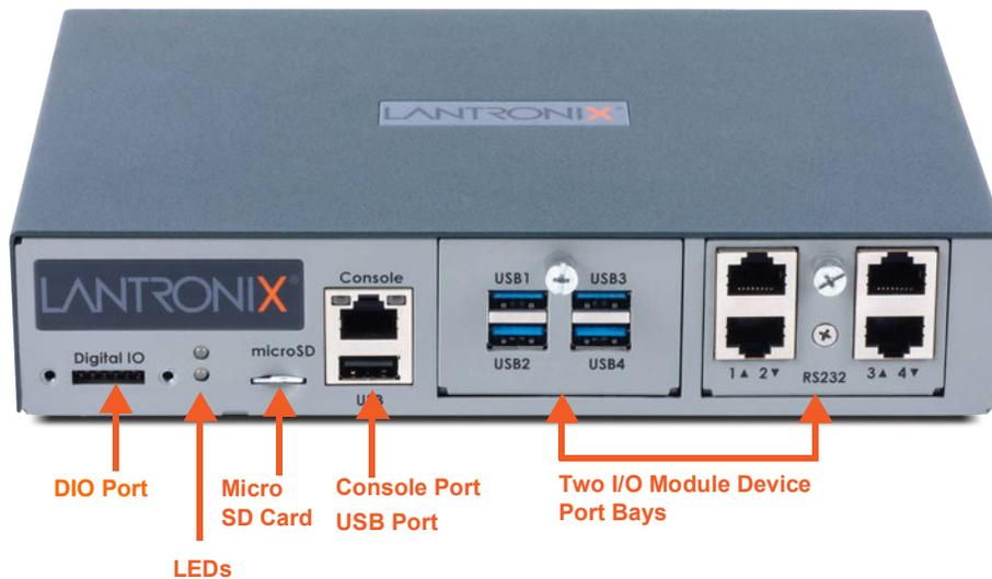
The appearance and function of the EMG unit will depend upon the type(s) of I/O modules installed in the bays.
