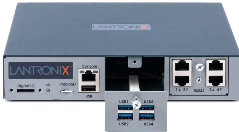
5. The module will sit flush with the EMG chassis.
