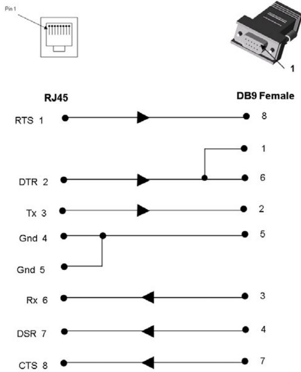
Use PN 200.2070A adapter with a PC's serial port.
