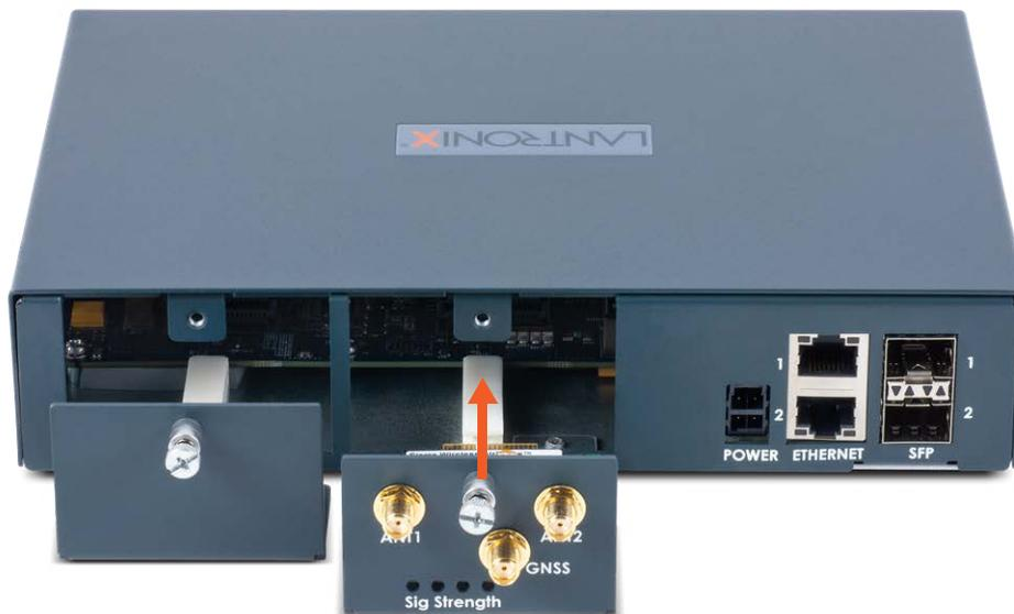
5. The module will sit flush with the EMG chassis.
