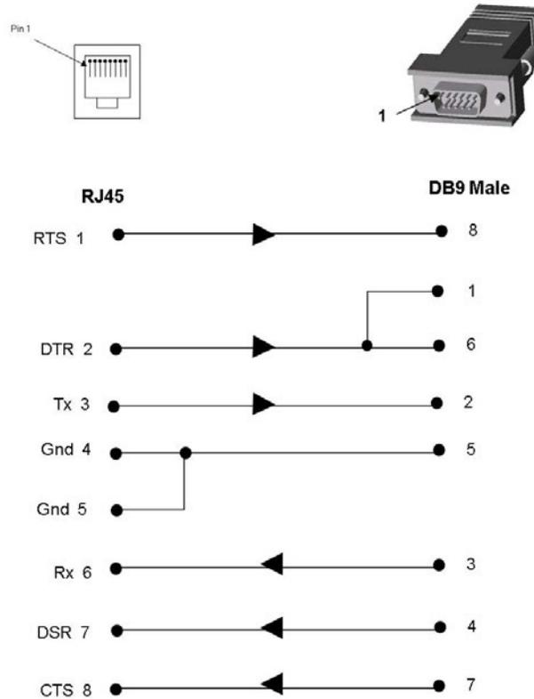
Figure C-4 RJ45 Receptacle to DB9F DCE Adapter for the EMG Unit (PN 200.2070A)
