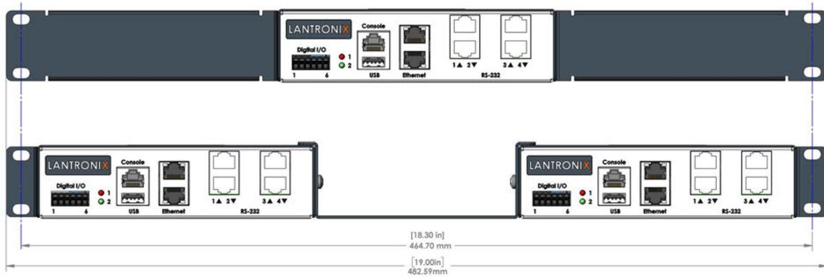
Figure 4-4 EMG 7500 Rack Mount Screw Placement
