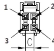
Figure 4-10 EMG 7500 Cellular Module Power Input
