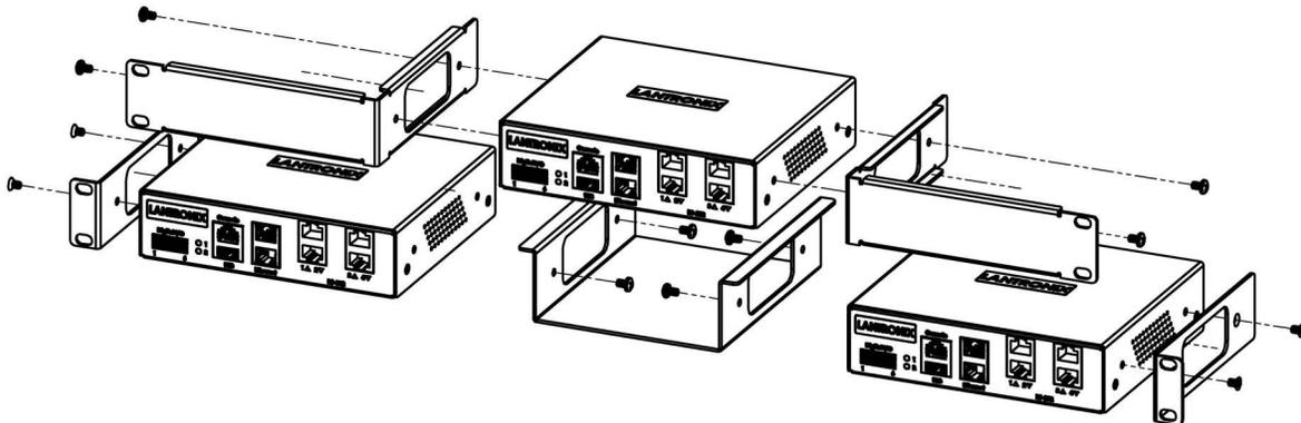
1. Attach the brackets on the sides of the EMG unit using a screwdriver and the screws provided with the mounting kit.
