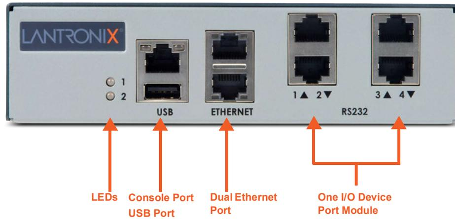
The appearance and function of the EMG unit will depend upon the type of I/O module installed.
