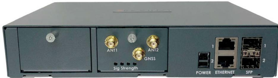
6. Tighten the screw on the module with your fingers. Be careful not to over tighten it.
