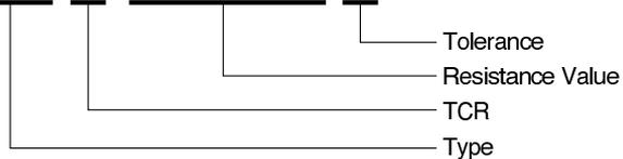
Resistance value, in ohm, is expressed by a series of six characters, five of which represent significant digits. R or K is a dual-purpose letter that designates both the value range (R for ohmic; K for kilo-ohm) and the location of decimal point.
