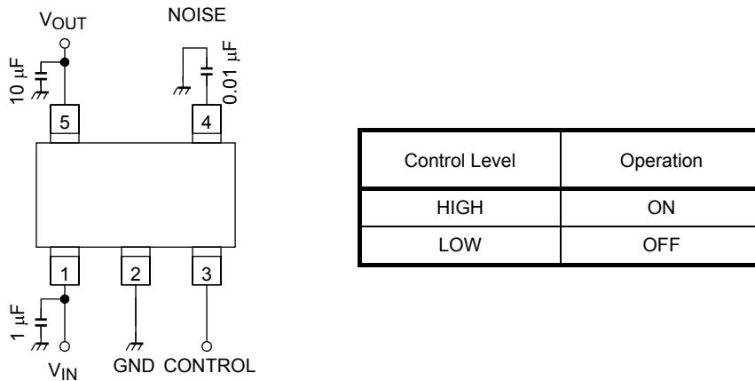
The figure above shows the recommended configuration for using a point regulator. Insert a capacitor for stable input/output operation.
